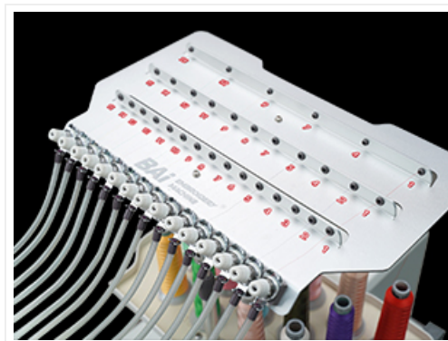
Figure 4: Threading Guide. This close-up image shows the upper threading path of the embroidery machine, indicating the
