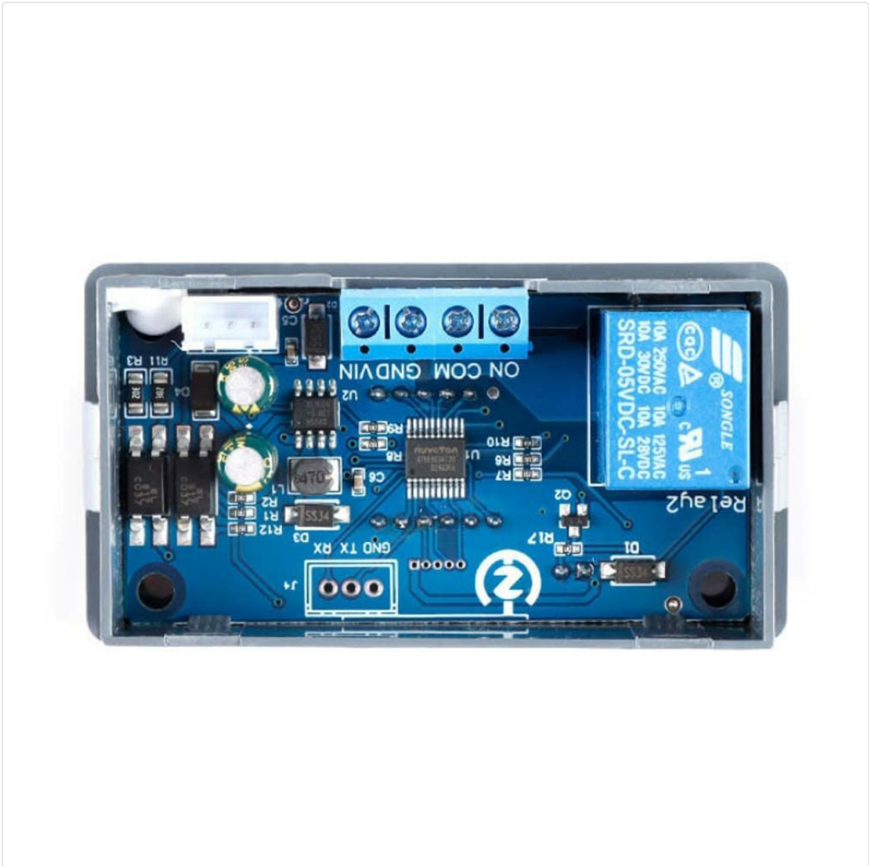
Figure 3: Back view of the ZK-KTD2 module. This image displays the reverse side of the module, revealing the printed circuit board (PCB), the Songle SRD-05VDC-SL-C relay, and various electronic components. Screw terminals for power input (GND, VIN) and relay output (ON, COM, GNDVIN) are visible, indicating connection points for power and controlled devices.
