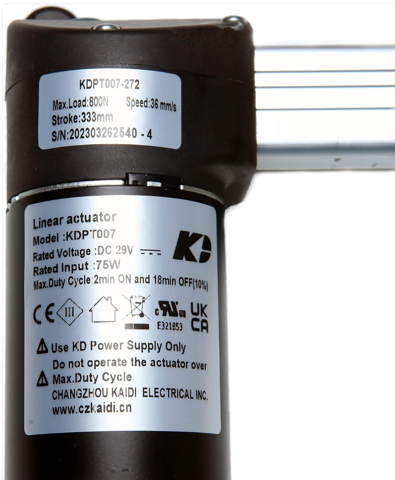
Image 2.1: Close-up view of the Kaidi motor label. This label displays critical information such as the model number (KDPT007-272), maximum load (800N), stroke length (333mm), rated voltage (DC 29V), rated input (75W), and duty cycle warnings. Always refer to this label for specific operational parameters and safety guidelines, including the instruction to use only a KD Power Supply.
