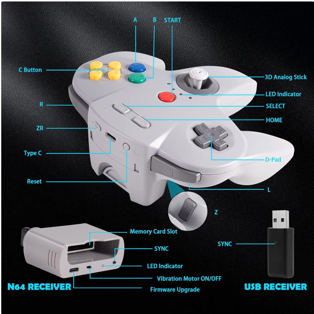
Figure 2: Detailed diagram illustrating the controller's buttons (C Button, R, ZR, 3D Analog Stick, LED Indicator, SELECT, HOME, D-Pad, L, Z, START, A, B), Type C charging port, Reset button, and the SYNC buttons on both the N64 Receiver and USB Receiver.
