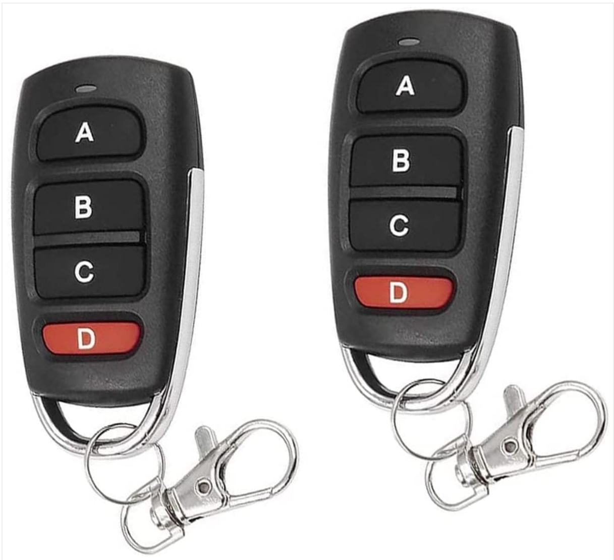
Figure 1: Bkiyougo Universal Duplicator Remote Controls. These remotes are designed for cloning existing 433.92 MHz fixed and learning code remotes.
