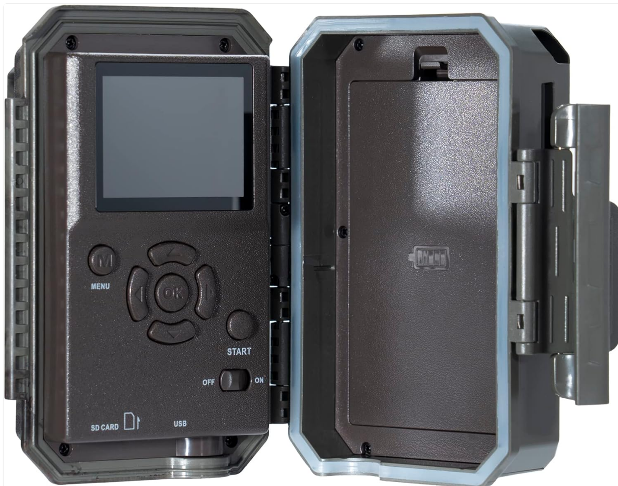
Figure 8: The 2.4-inch color display and control buttons for menu navigation.
