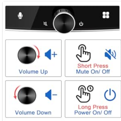
Figure 4: Rotating knob functions for volume and power.
