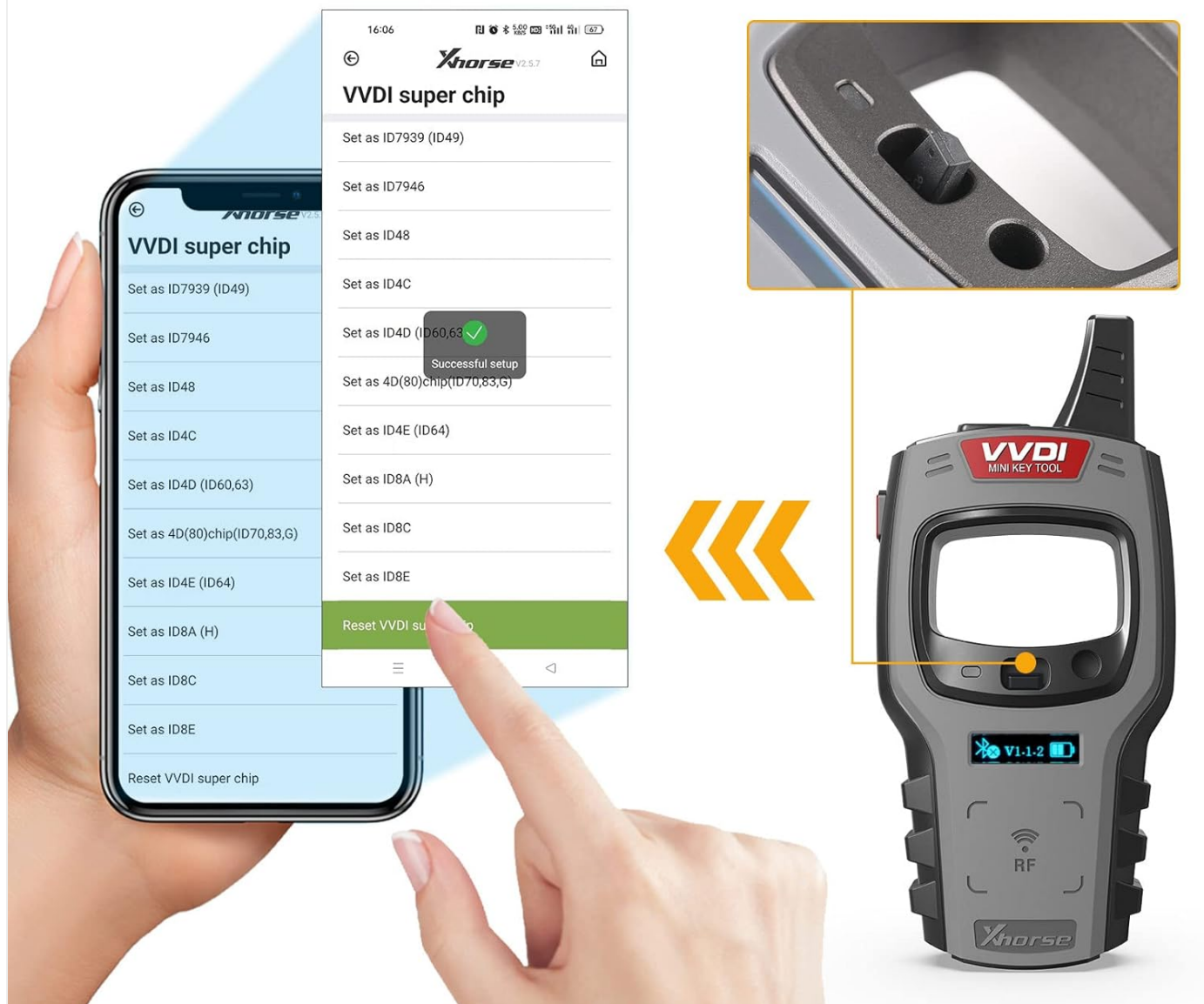
Figure 7: Interface for setting/renewing VVDI Super Chips to different ID types.
