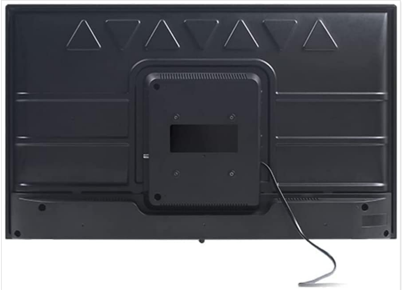
Rear view of the TV, highlighting the VESA mounting area.
