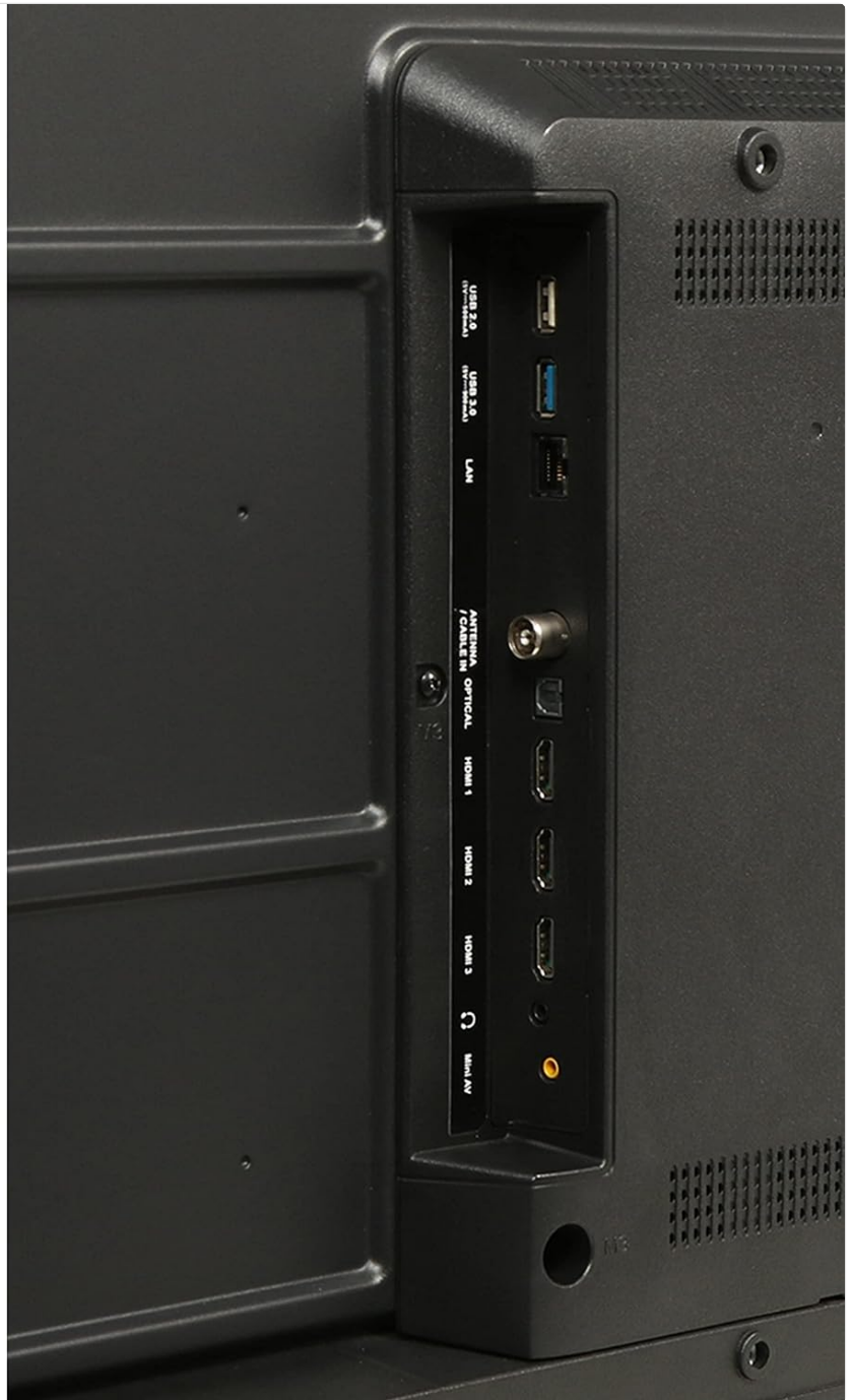
Figure 3: Detailed view of the television's connectivity ports.
