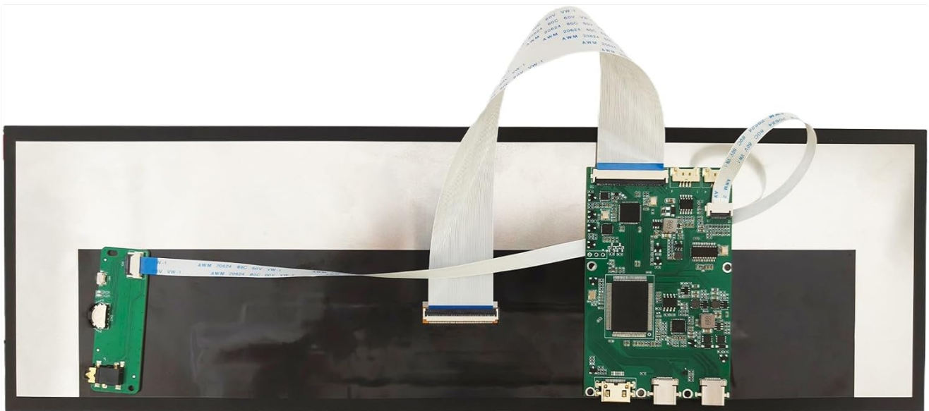
Image 4.1: The LCD panel connected to the controller board via the signal cable.
