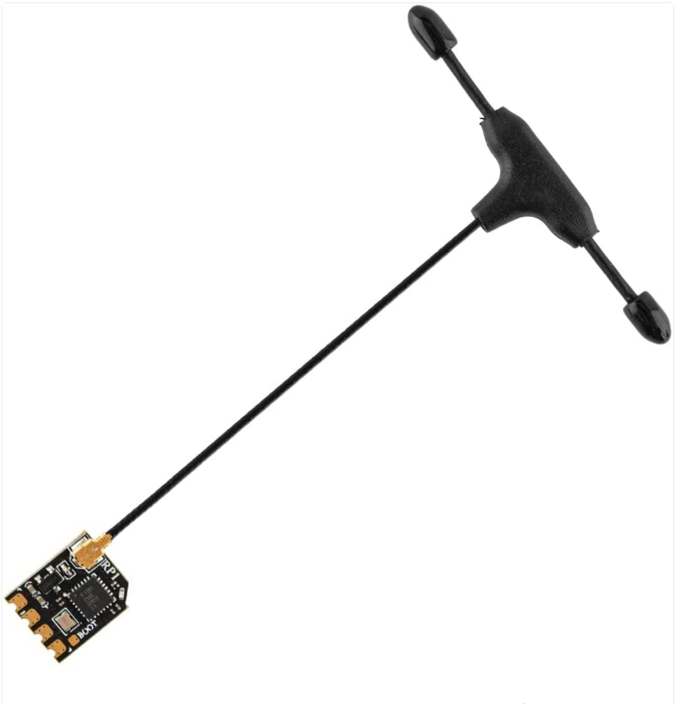
Image 4.4: The RP1 receiver with the 65mm UFL T antenna properly connected, ready for installation into a model.
