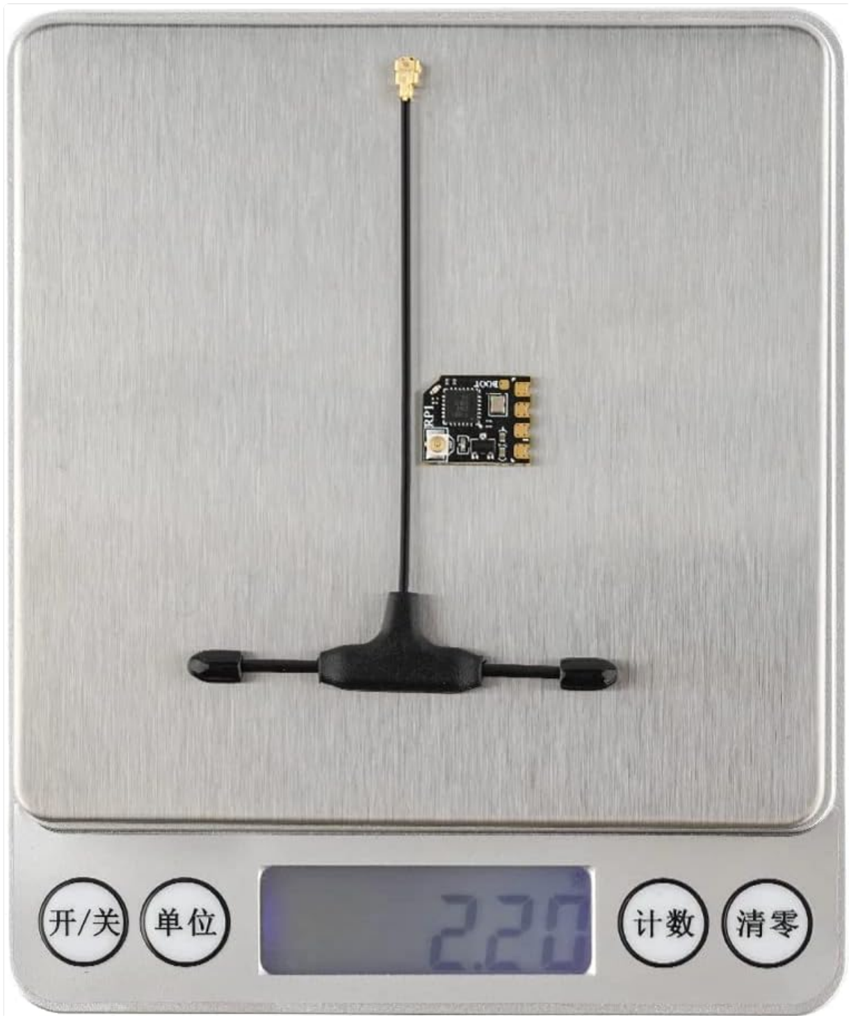
Image 3.2: The RP1 receiver with its T antenna, demonstrating a combined weight of approximately 2.20 grams on a digital scale.
