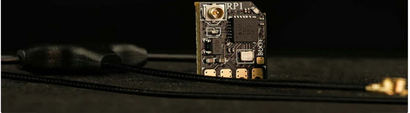
Image 1.1: The RadioMaster RP1 ELRS Serial Receiver, highlighting its suitability for whoops, drones, and fixed-wing aircraft, along with its low latency and high refresh rate capabilities.
