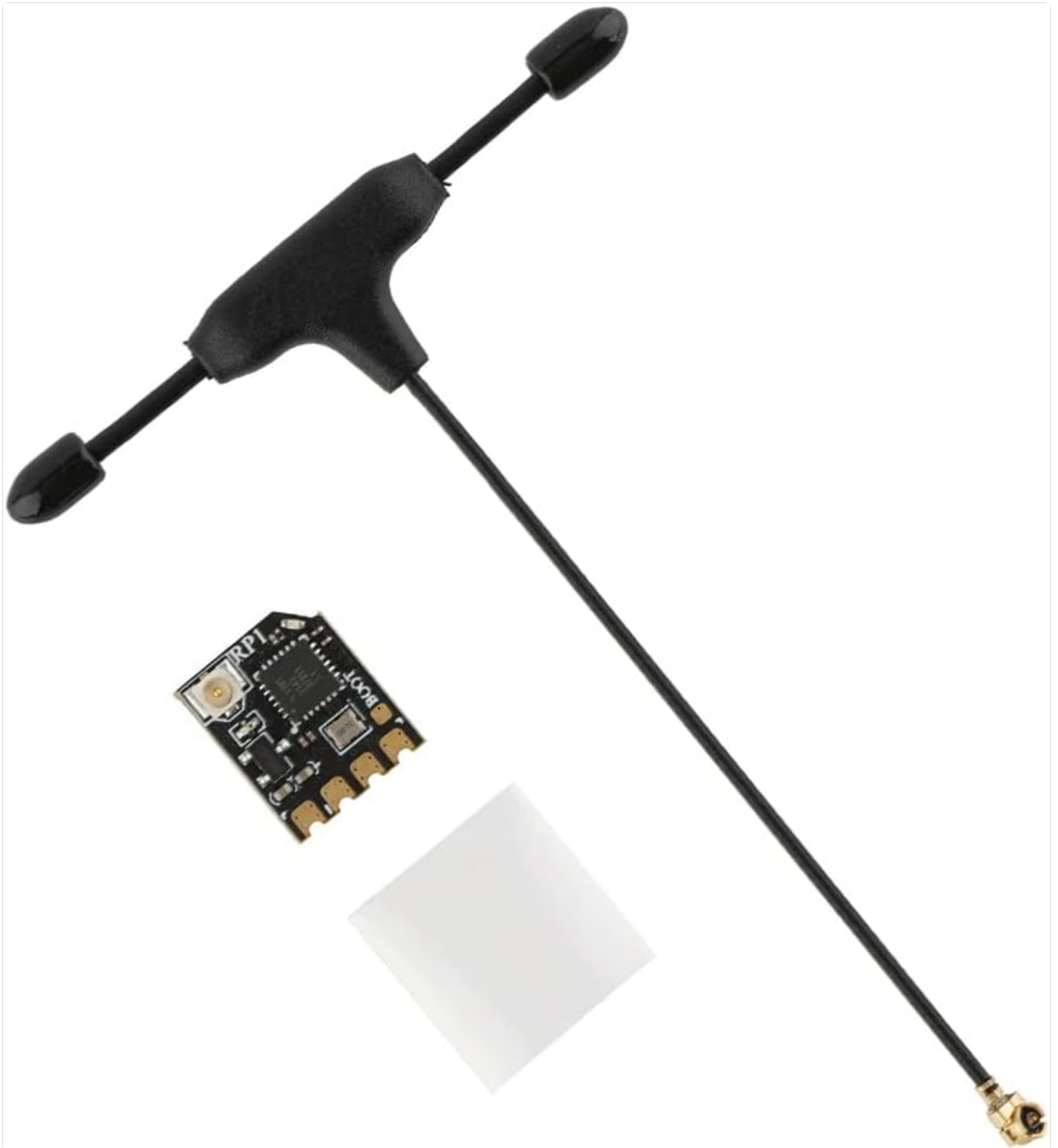
Image 2.1: The complete package contents, showing the RP1 receiver, the 65mm UFL T antenna, and a piece of heat shrink tubing.
