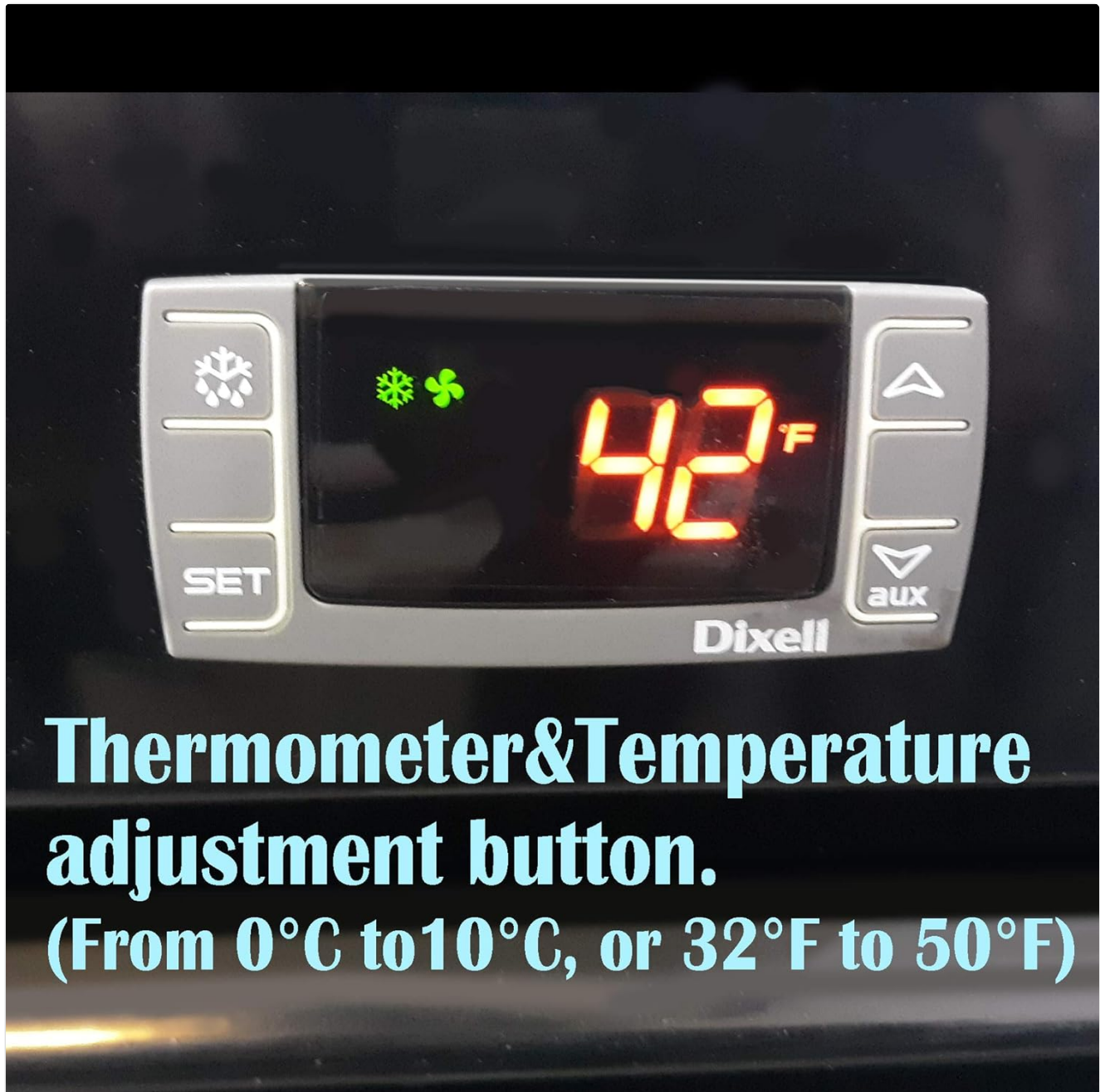
Image 4.1: Dixell digital thermometer display and temperature adjustment buttons, showing a reading of 42°F.
