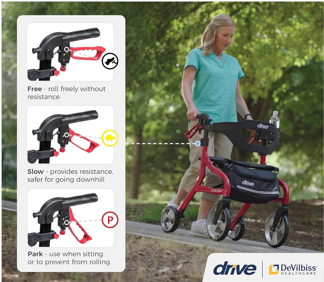
Figure 4: Braking System Modes
