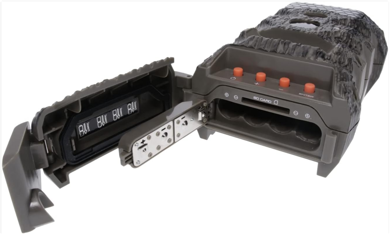
The camera's interior, with the side panel open, revealing the battery compartments and the SD card slot.
