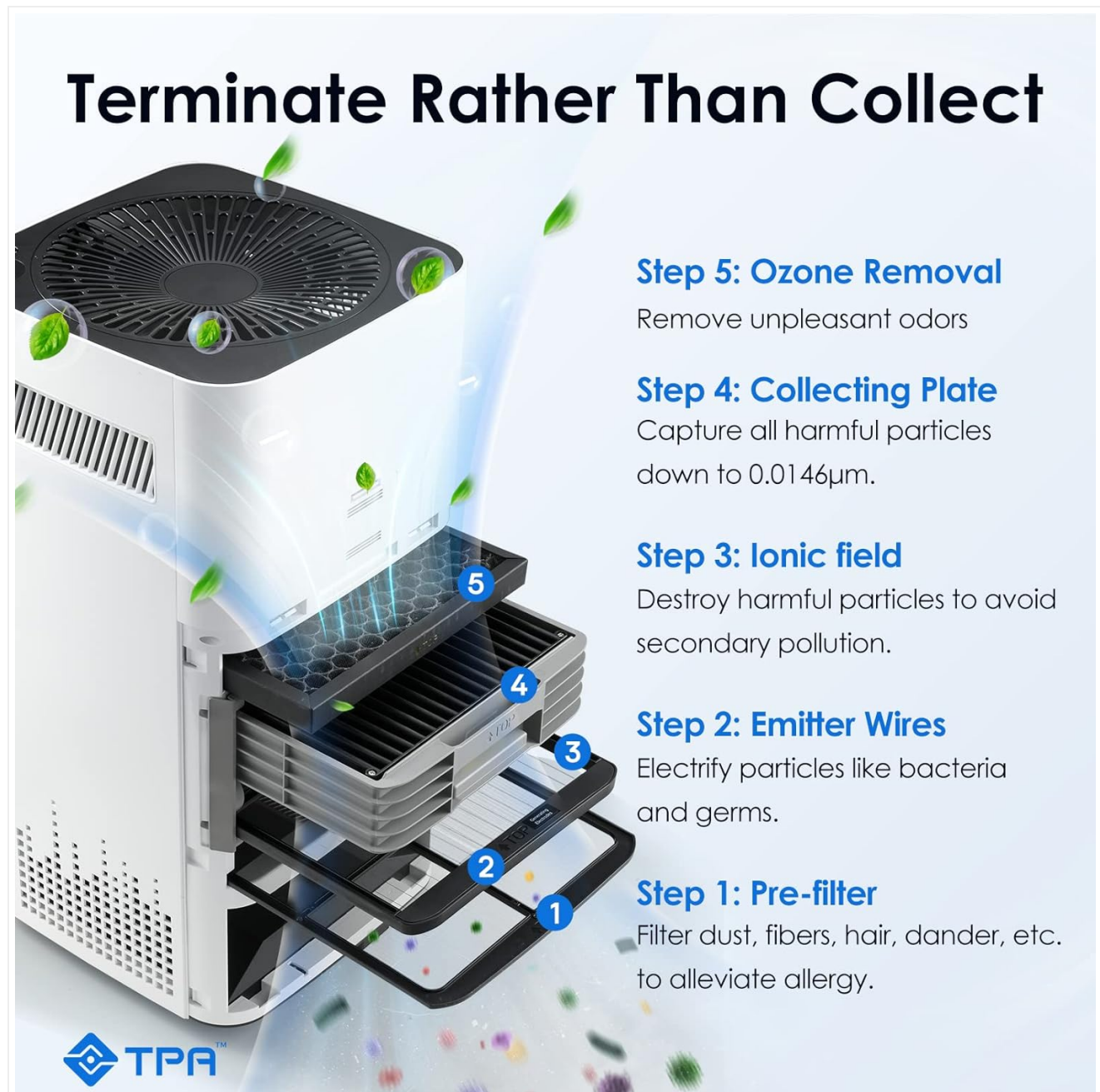
Image 3.1: Airdog X3 Filtration System Layers.
