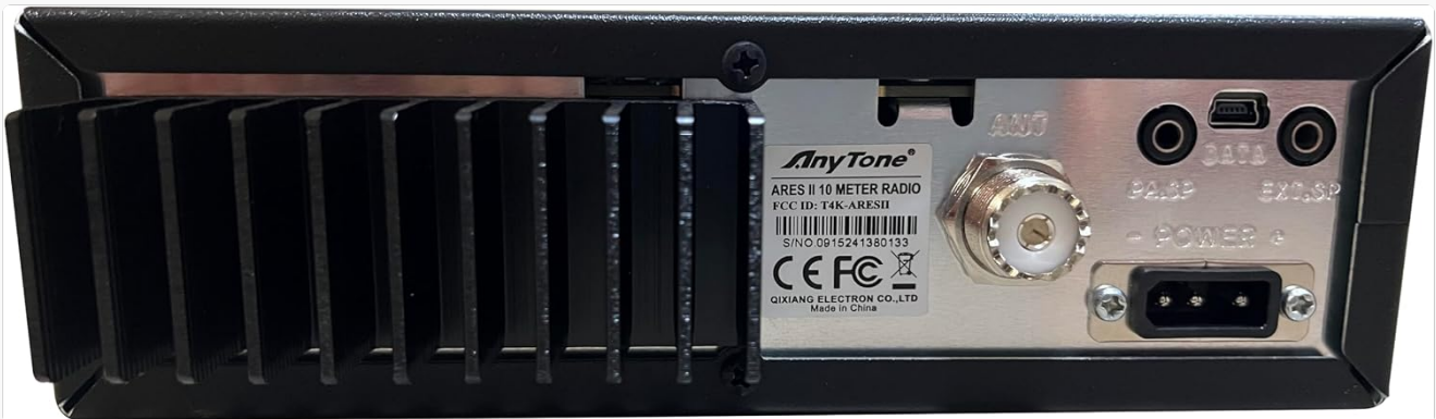
Image: Detailed view of the AnyTone ARES II rear panel, showing the antenna jack, power supply jack, PC programming port, and external speaker/PA jacks.
