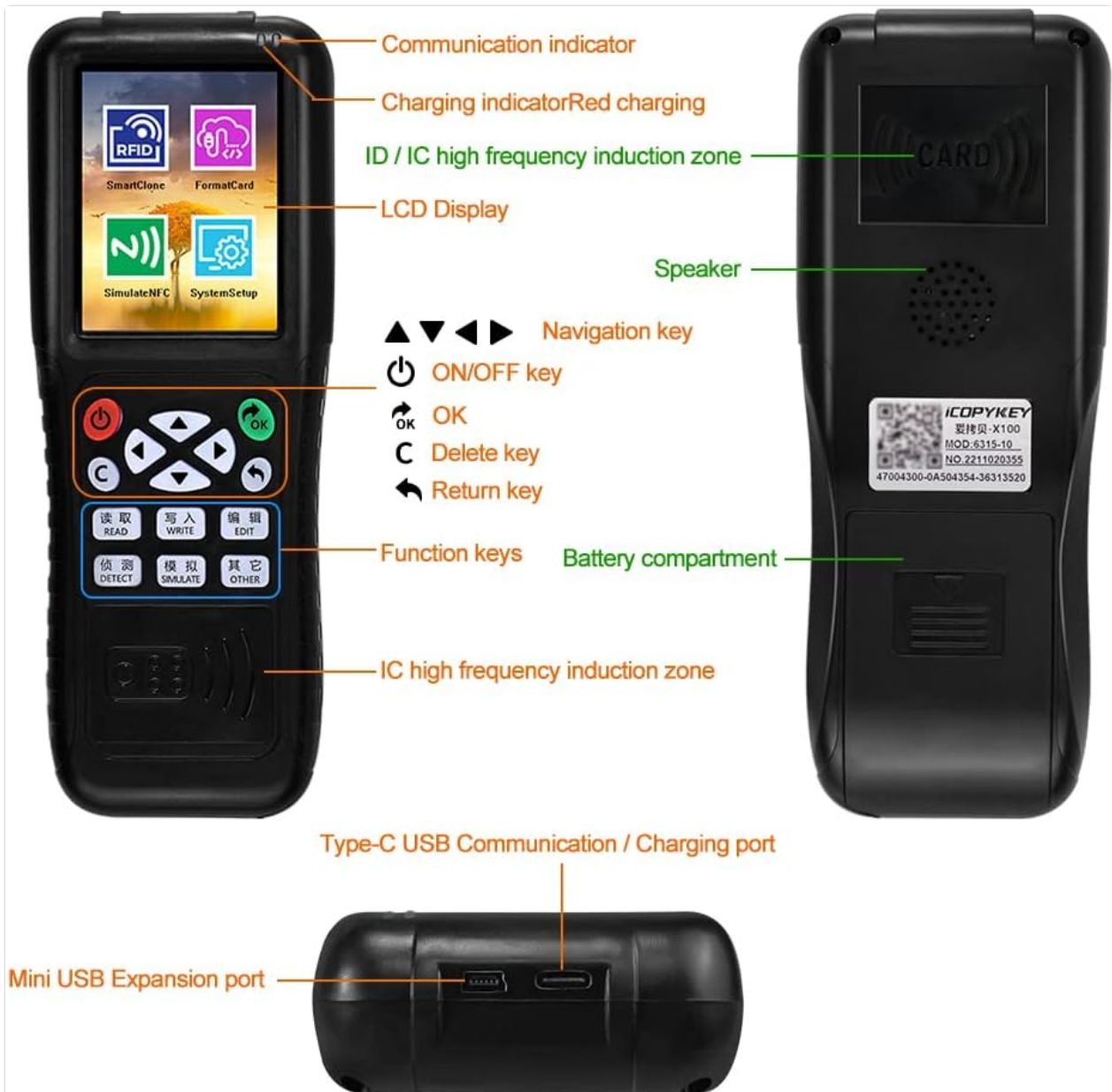
Image 2.1: Overview of the jasugKEY RFID Card Copier with labeled components including communication indicator, charging indicator, ID/IC high frequency induction zones, LCD display, speaker, navigation keys, function keys, battery compartment, Type-C USB port, and Mini USB expansion port.
