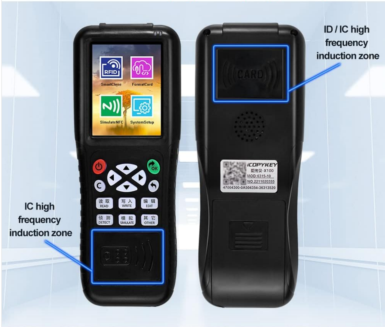
Image 2.2: Illustration of the dual induction areas on the jasugKEY RFID Card Copier, highlighting the ID/IC high frequency induction zones on both the front and rear of the device.
