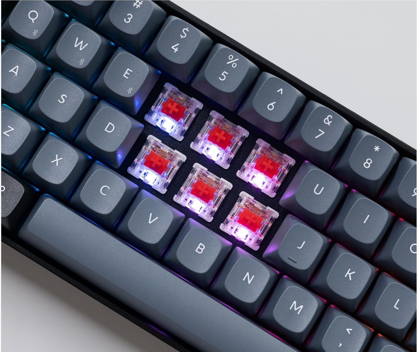
Image: Close-up of the Keychron K12 Pro keyboard showcasing its RGB backlighting illuminating the hot-swappable switches beneath the keycaps.
