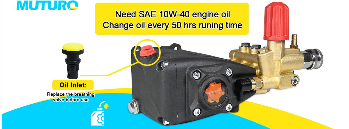
Figure 6: Oil inlet and oil change recommendations.
