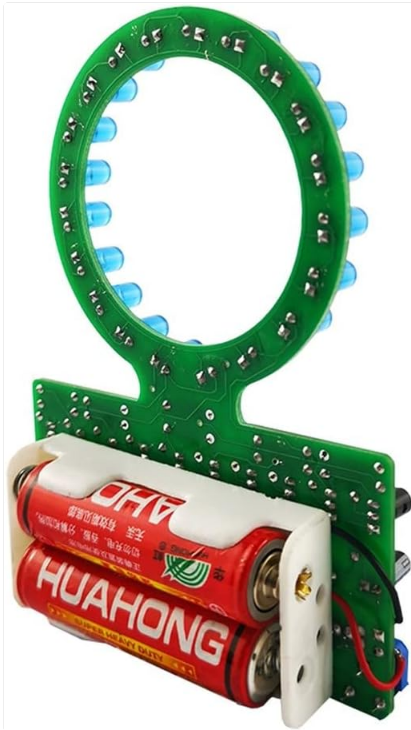
Image 5.1: The assembled circuit board with two AA batteries correctly installed in the battery holder, ready for operation.
