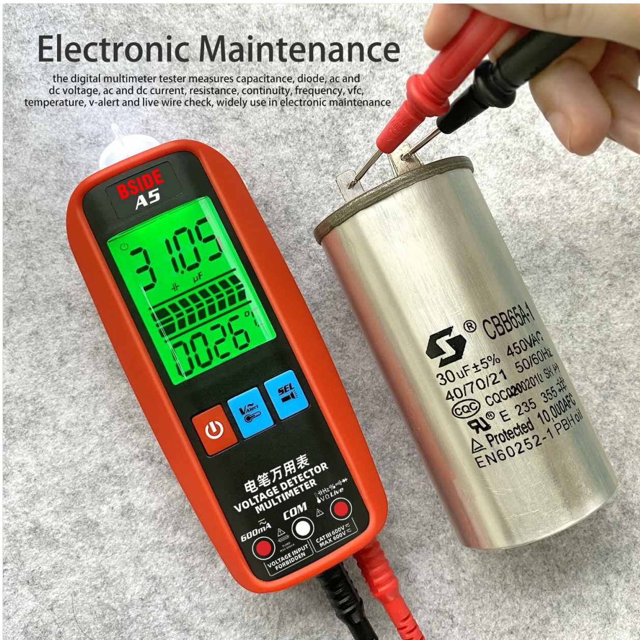
Image 4.1: The multimeter is a versatile tool for electronic maintenance, including capacitance testing.
