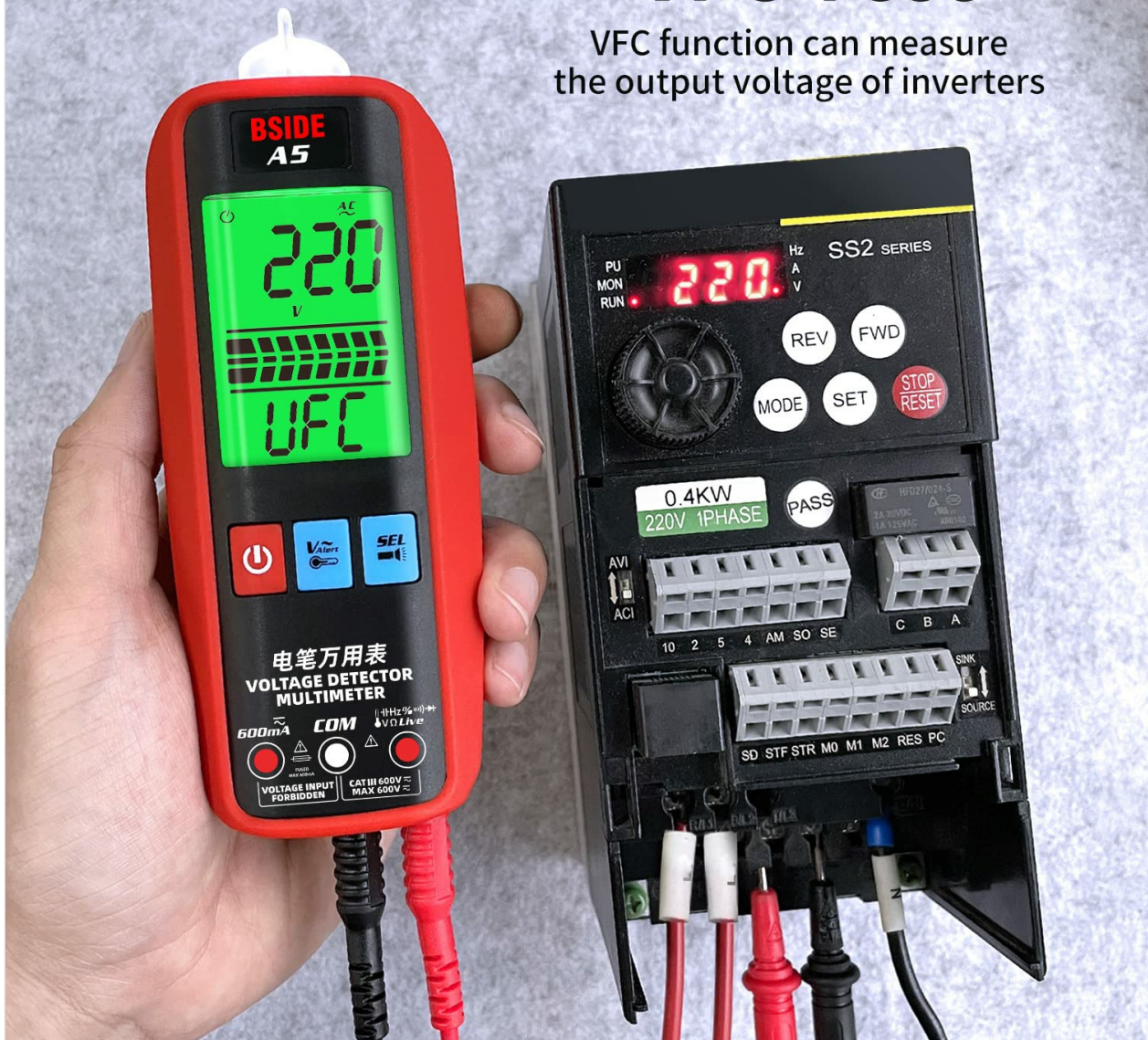
Image 3.4: The VFC mode measures the output voltage of inverters, displaying the voltage and frequency.
