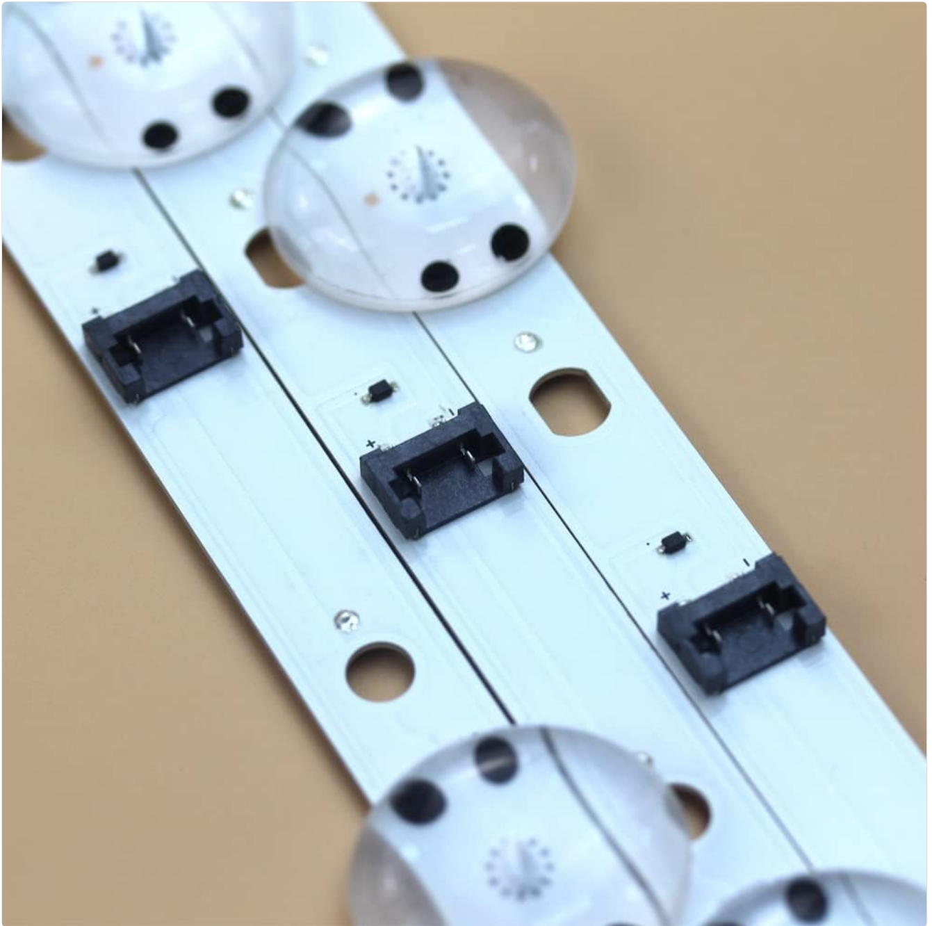
Image 3.3: A close-up of the black electrical connectors on the backlight strip, which are used to link the strips together and connect them to the TV's power supply. Ensure these connectors are securely fastened.
