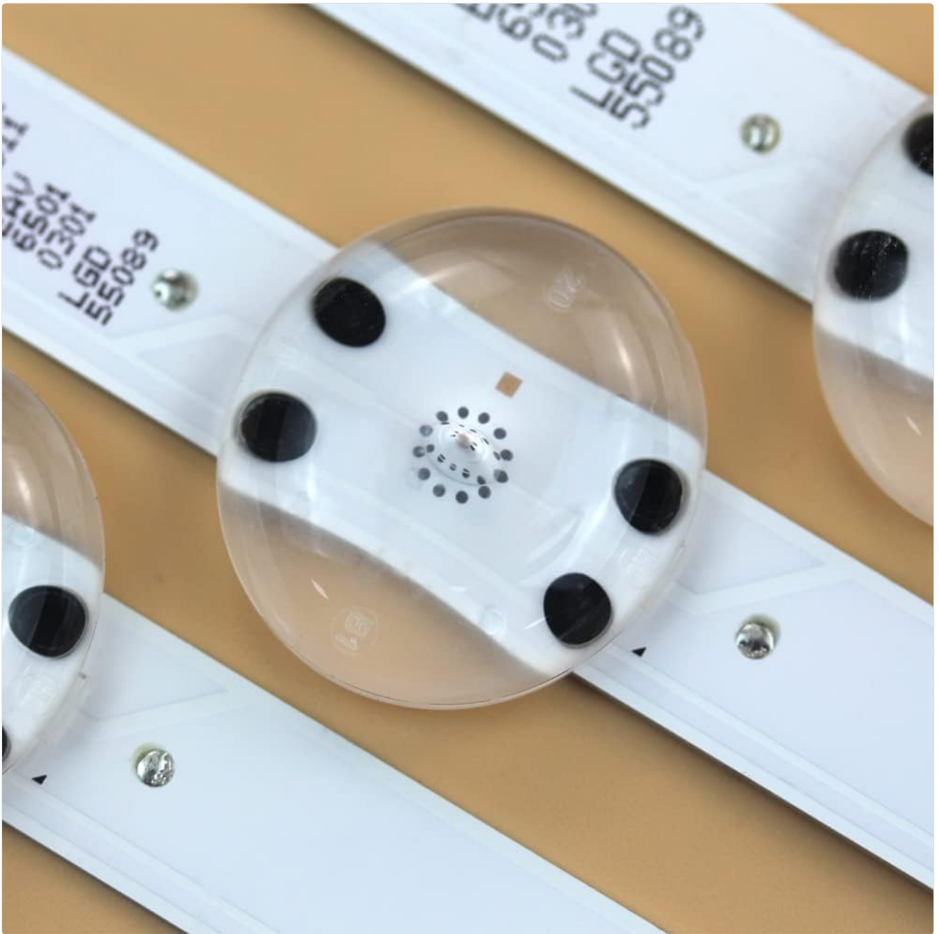
Image 3.2: A detailed view of an individual LED lens on the backlight strip, showing the clear dome and the underlying LED components. This design ensures optimal light diffusion.
