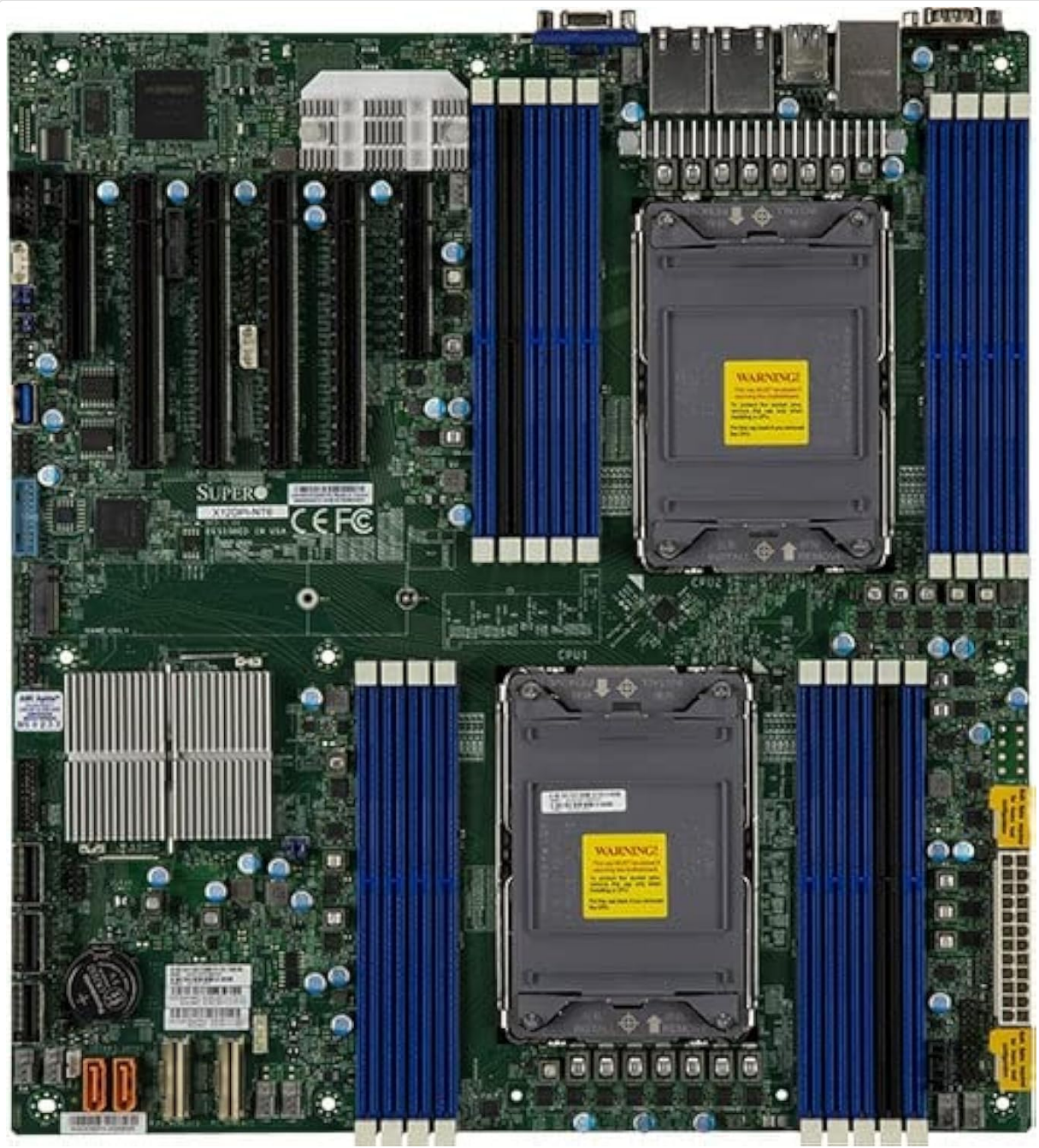
Figure 1: Top-down view of the Supermicro MBD-X12DPI-N6-B E-ATX Server Motherboard, showcasing its dual LGA 4189 CPU sockets, 18 DDR4 DIMM slots, multiple PCIe 4.0 expansion slots, and various connectors for storage and peripherals. The board features a green PCB with blue and black DIMM slots, and silver heatsinks for chipset and VRMs.
