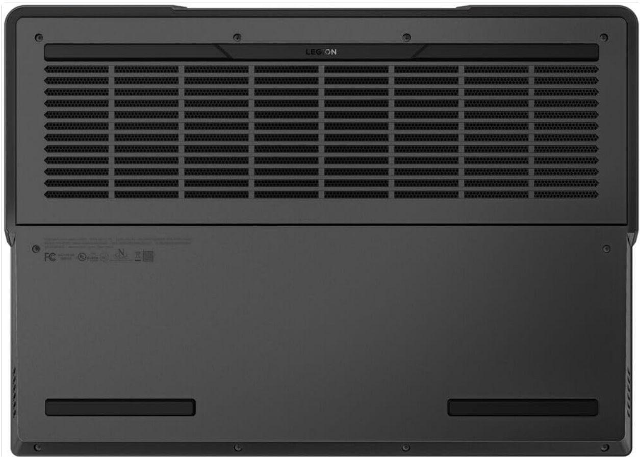
Image 4.1.1: Bottom view of the laptop, illustrating the large ventilation areas crucial for cooling.
