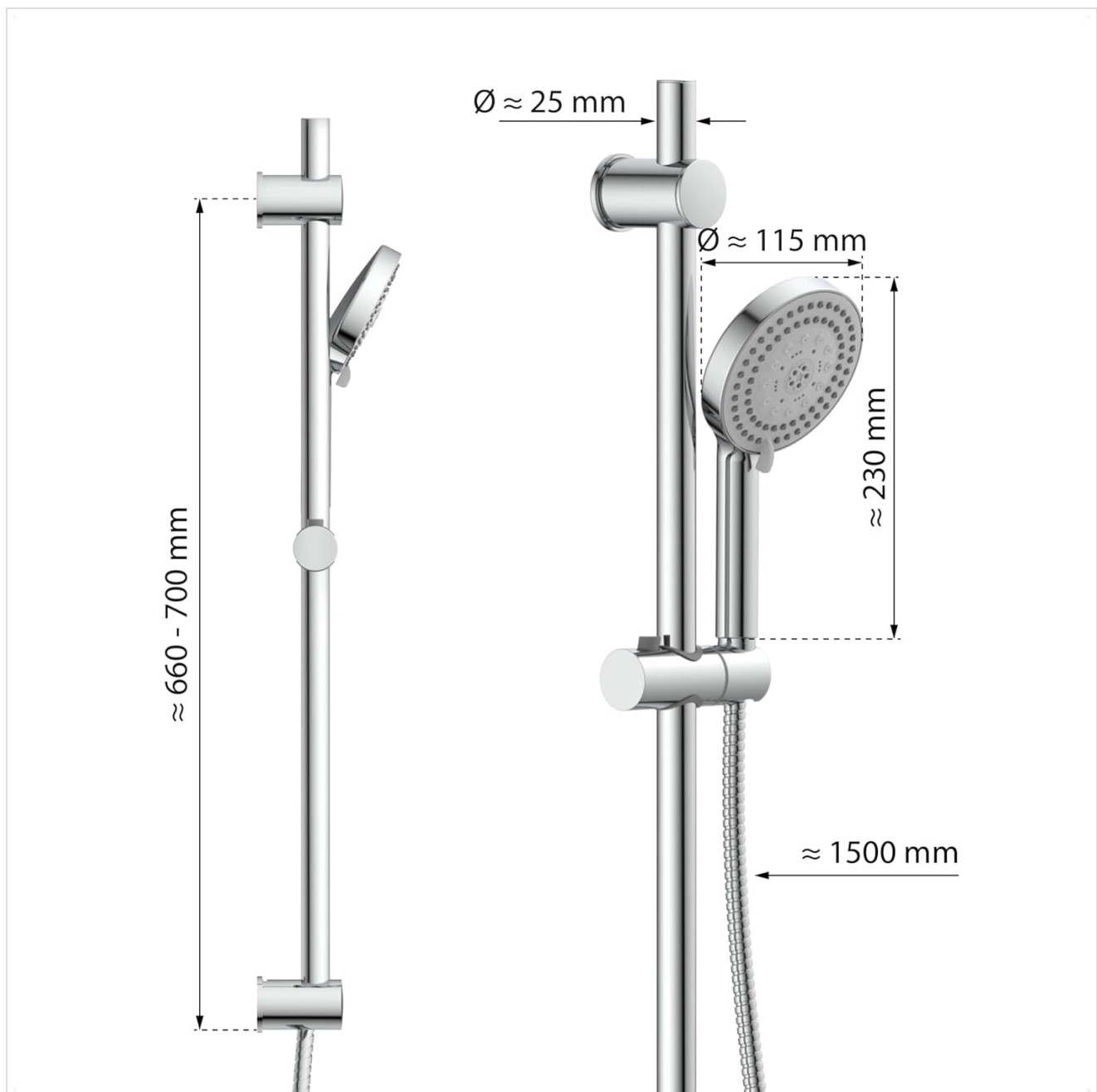
Image 3.2: Detailed dimensions of the EISL DX5082CSB shower rail set, including rail length (660-700mm), shower head diameter (approx. 115mm), and hose length (approx. 1500mm).
