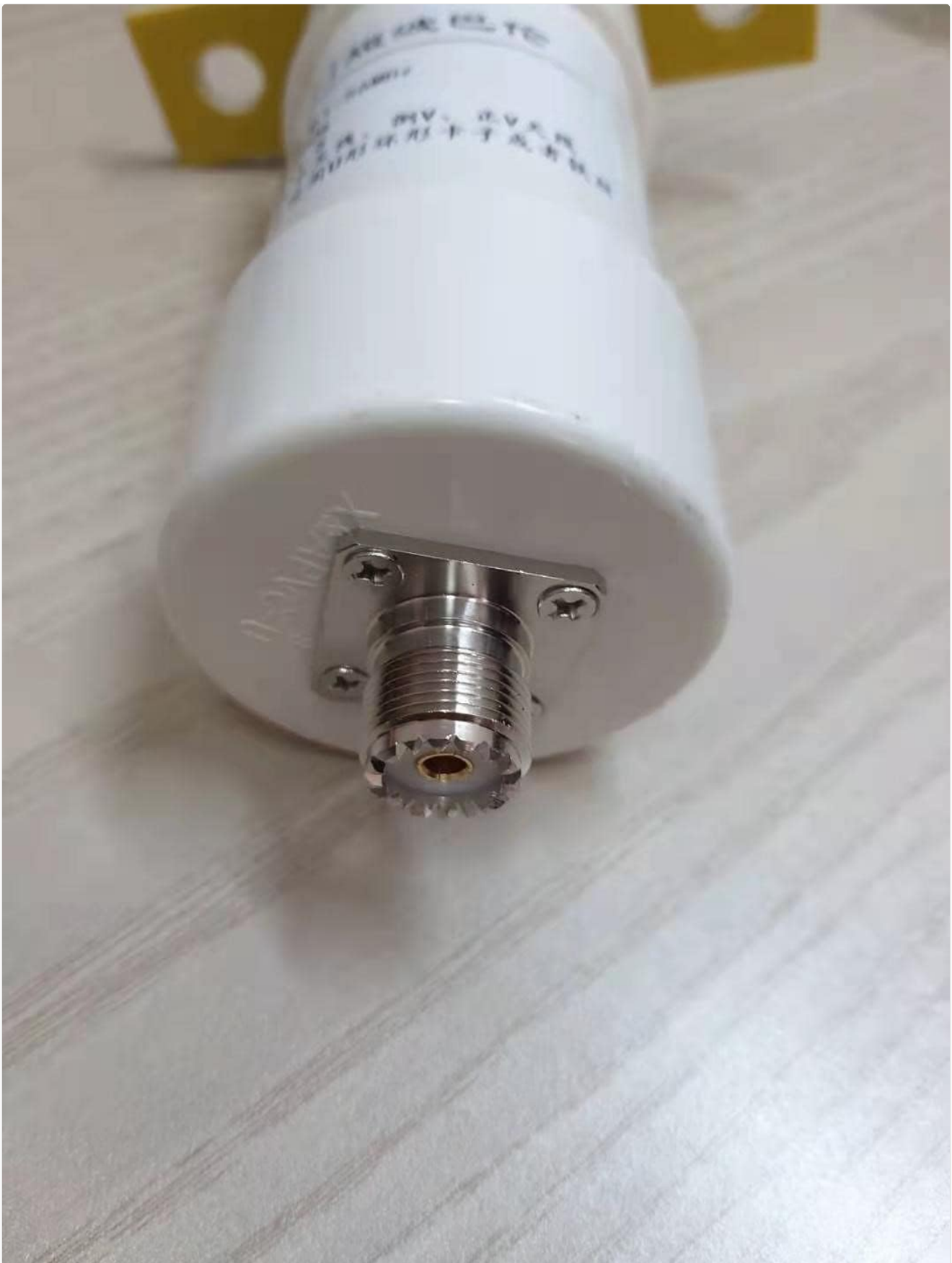
Figure 3: Bottom view with coaxial connector. This image shows the underside of the balun, clearly displaying the SL16-F (UHF Female) connector where the coaxial feedline is attached.
