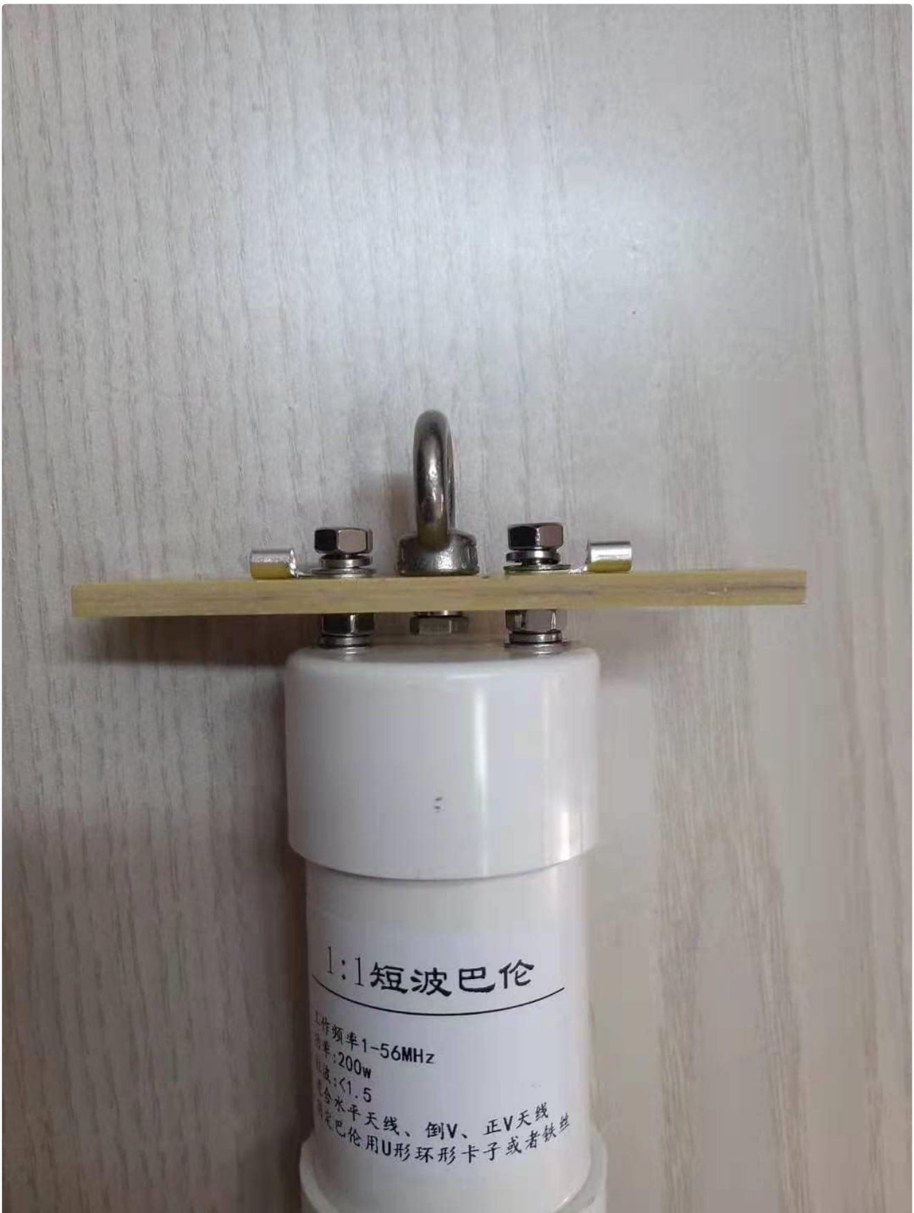
Figure 1: Top view of the balun with mounting points. This image displays the top section of the balun, highlighting the yellow mounting plate with two eye bolts for connecting antenna wires and a central metal eyelet for suspending the balun.
