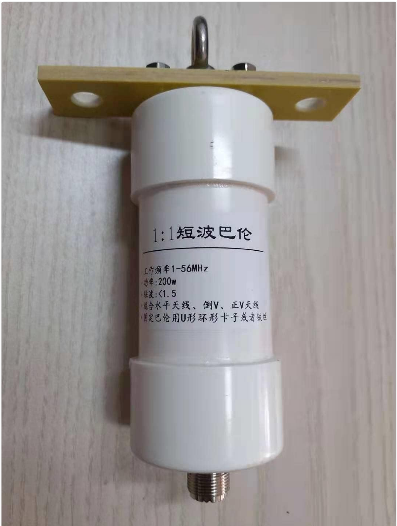
Figure 4: Complete balun assembly. This image presents a full view of the balun, showing both the top mounting bracket and the bottom coaxial connector, along with a label that includes specifications in Chinese.
