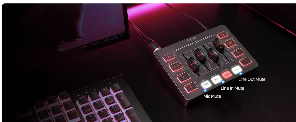
Figure 5.2: Mute buttons for various channels.
