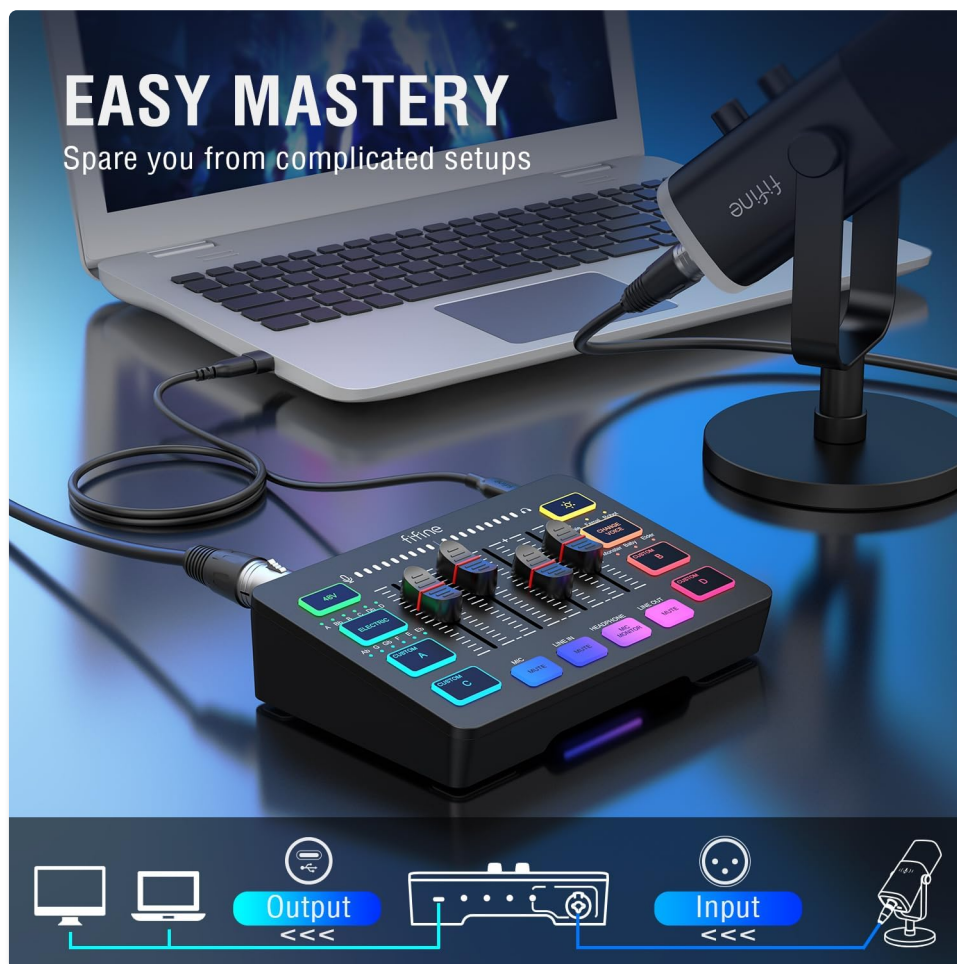
Figure 4.1: Connecting the mixer to a computer and microphone.
