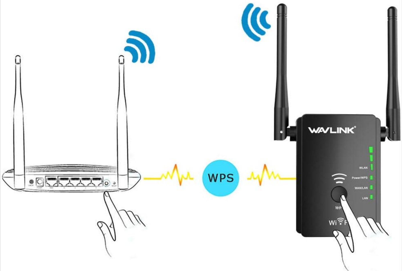
Figure 5: Easy installation using the WPS button.
