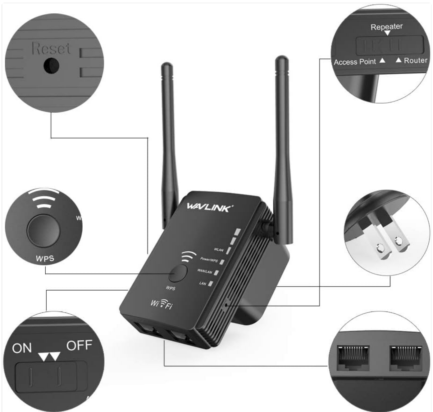
Figure 3: Key physical components and ports of the WAVLINK WiFi Extender.
