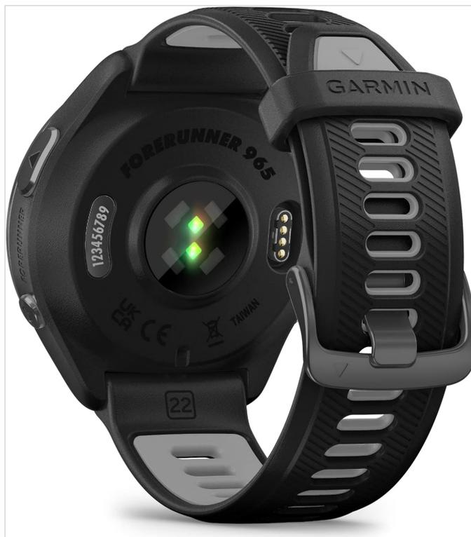
Figure 8: Back of the watch showing the optical heart rate sensors.
