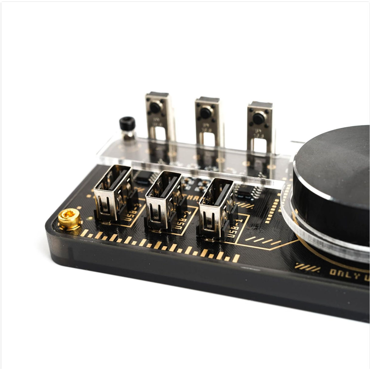
Figure 3: Close-up of the three USB 2.0 ports on the GeekHUB.
