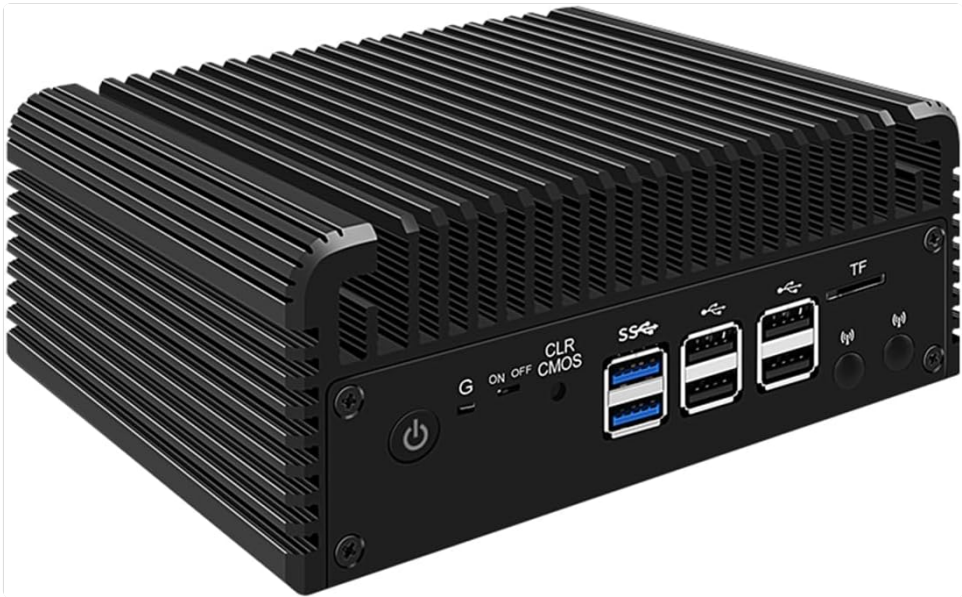
Figure 3.2: Front panel of the HUNSN RJ35. From left to right: Power ON/OFF button, G (indicator light), ON/OFF (indicator light), CLR CMOS button, two USB 3.0 ports (blue), four USB 2.0 ports (black), and a TF (MicroSD) slot. Two small holes for antennas are also visible.
