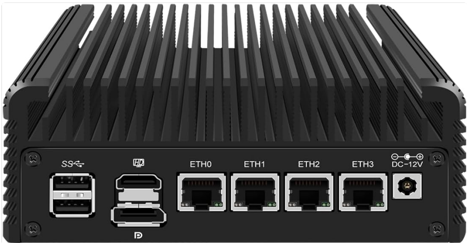
Figure 3.3: Rear panel of the HUNSN RJ35. From left to right: Two USB 3.0 ports (blue), HDMI 2.1 port, DisplayPort 1.4, four 2.5GbE LAN ports (ETH0, ETH1, ETH2, ETH3), and the DC-12V power input jack.
