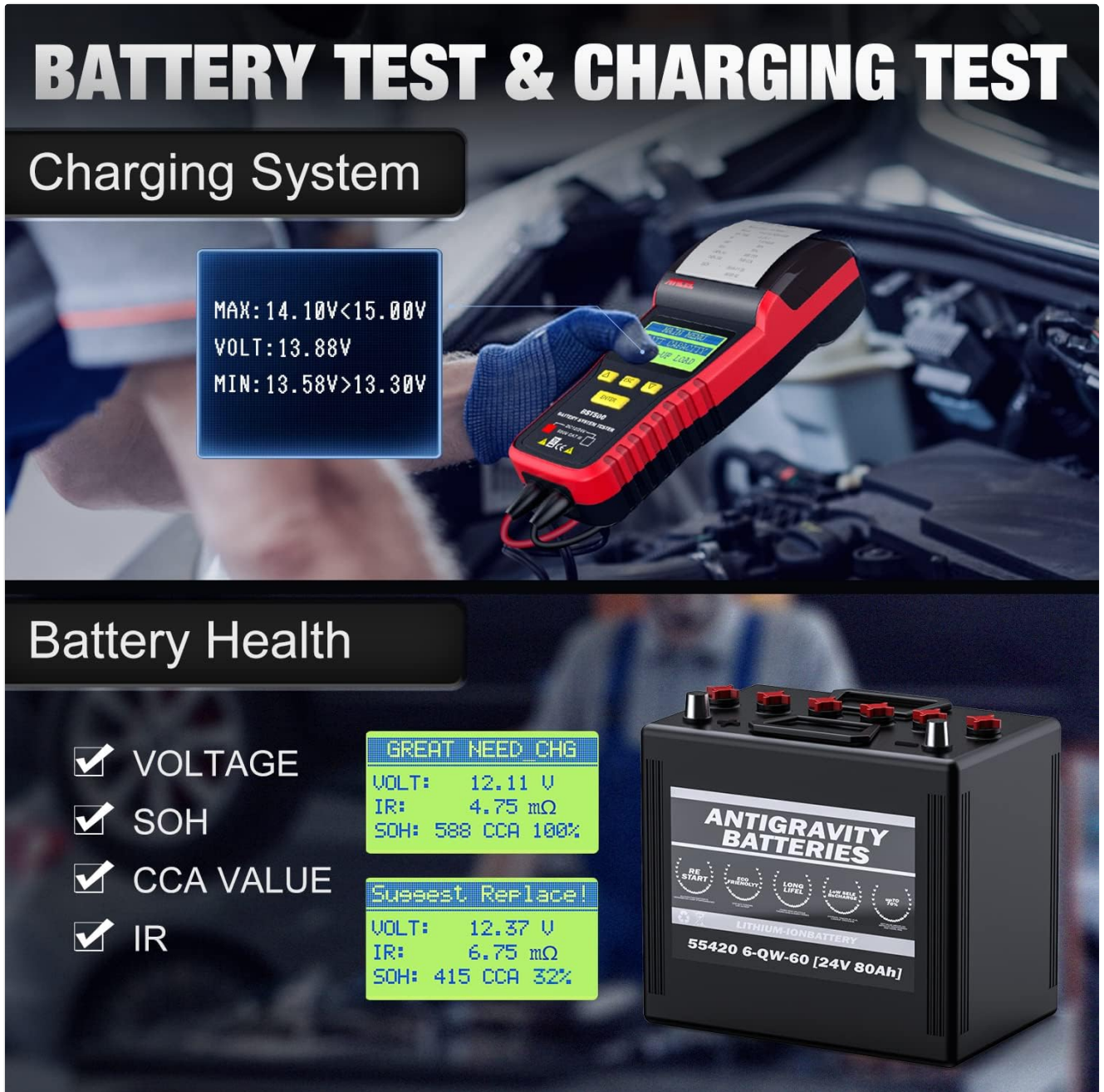
Image: The BST500 displaying results for Battery Health (Voltage, SOH, CCA Value, IR) and Charging System tests, showing detailed diagnostic information.
