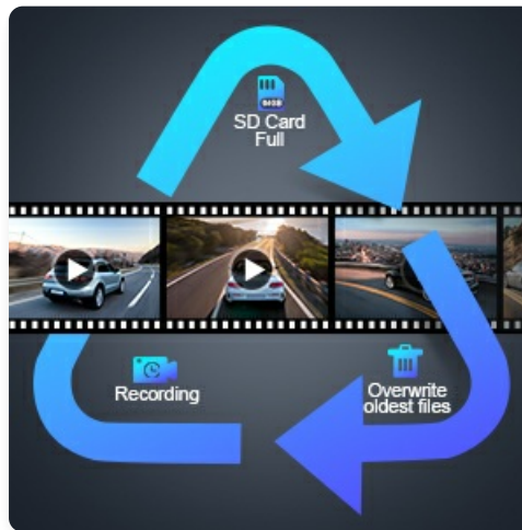
Image: A diagram illustrating the loop recording process, where the dash cam records, and when the SD card is full, it overwrites the oldest files.
