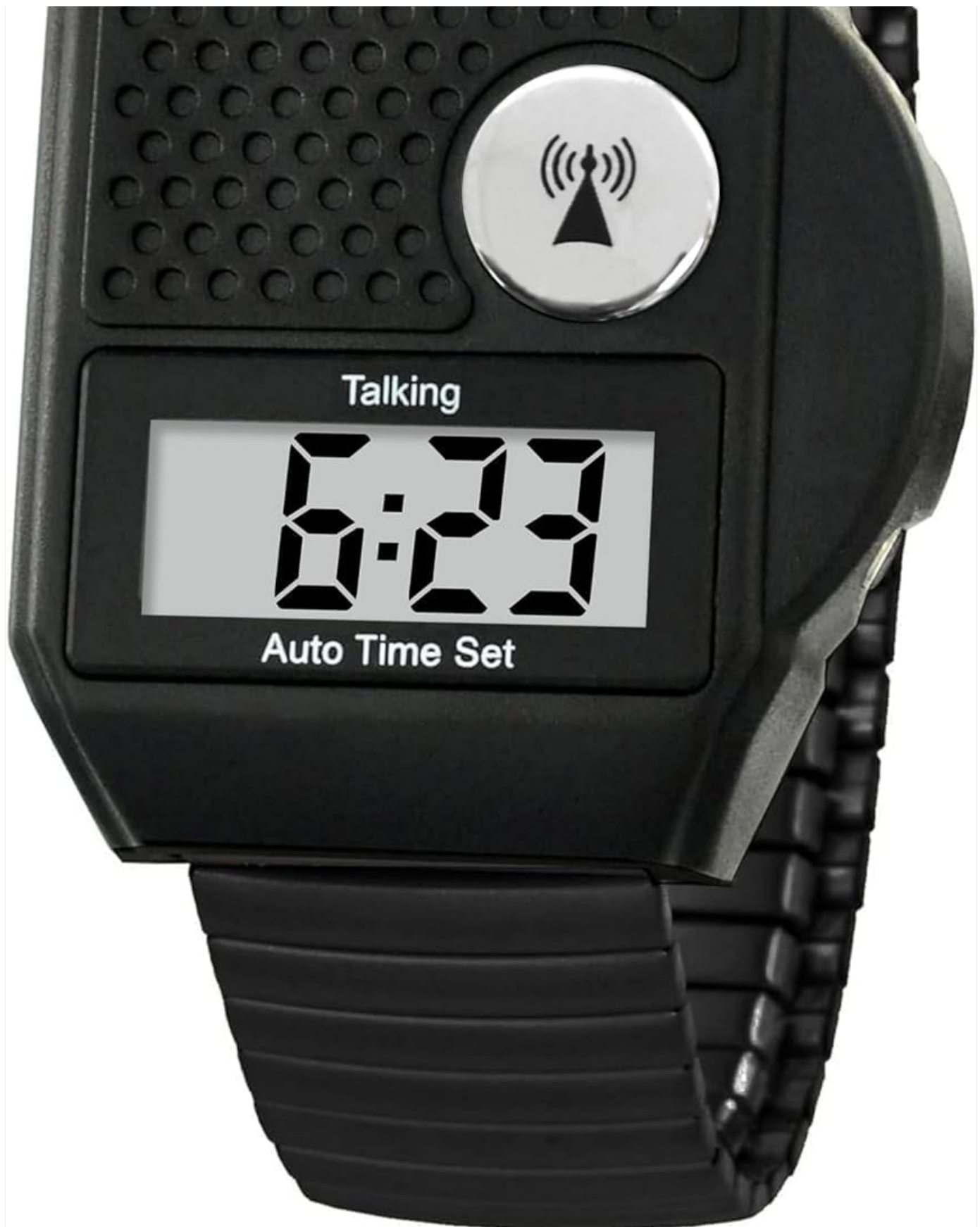
Image 4.1: Front view of the watch, highlighting the speaker and display.
