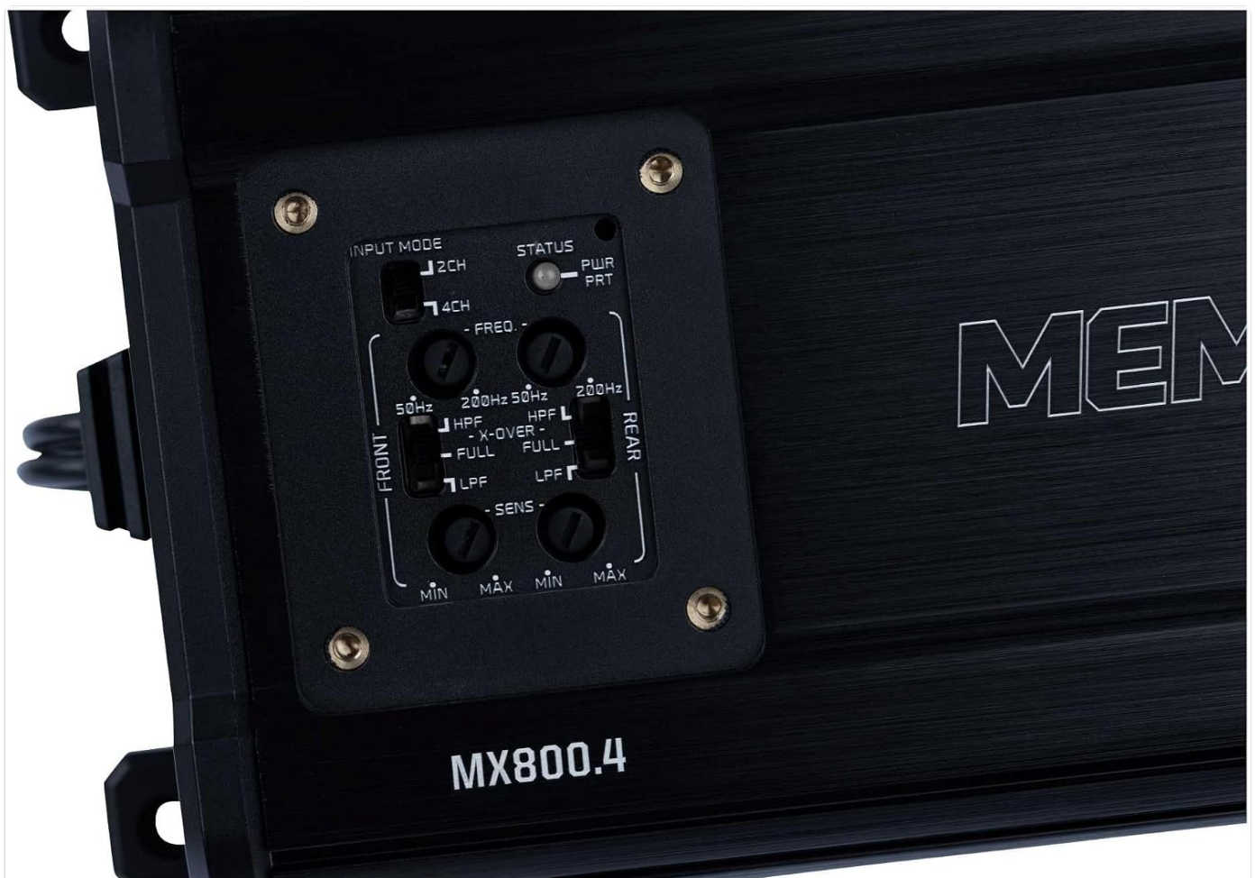
Image: Detailed view of the MX800.4's top-mounted control panel, showing switches for input mode, frequency crossovers (HPF/LPF/FULL), and sensitivity (SENS) adjustments for both front and rear channels.
