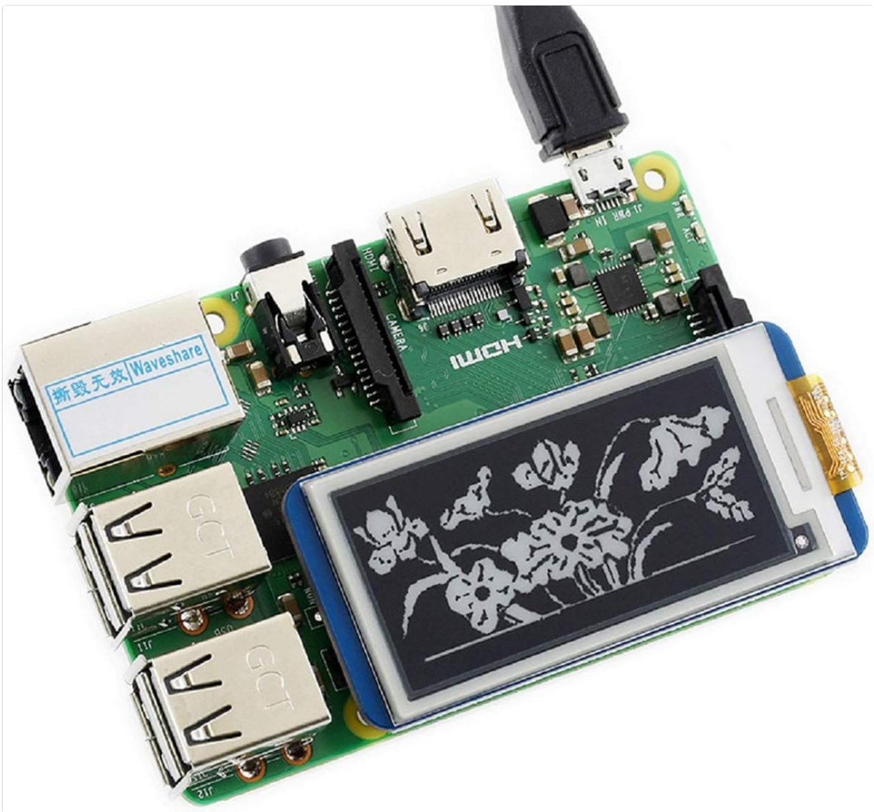
Figure 3: The 2.13inch E-Paper HAT correctly installed on a Raspberry Pi board, demonstrating its compact integration.
