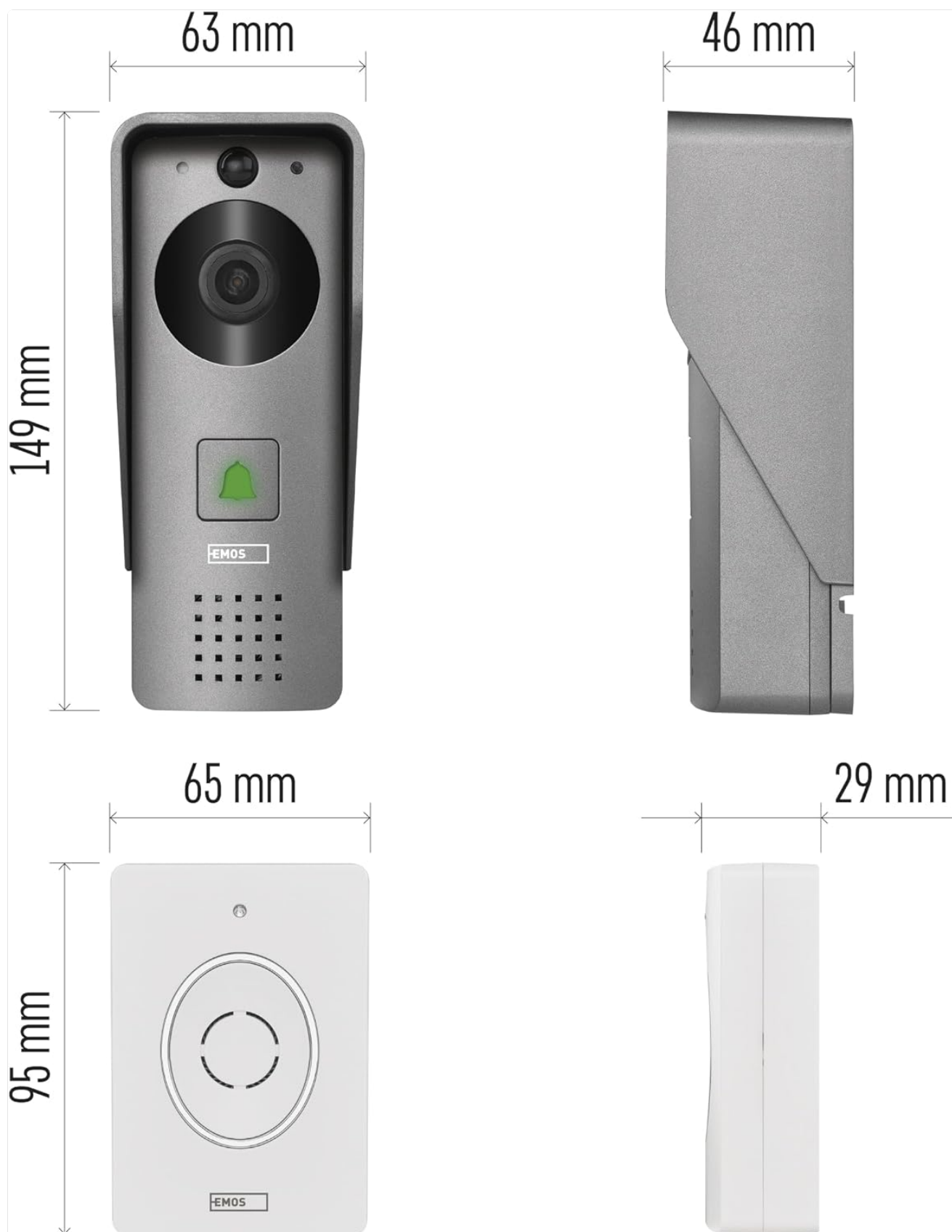
Figure 7.1: Dimensions of the EMOS GoSmart IP-09D CLOC video doorbell and indoor chime.
