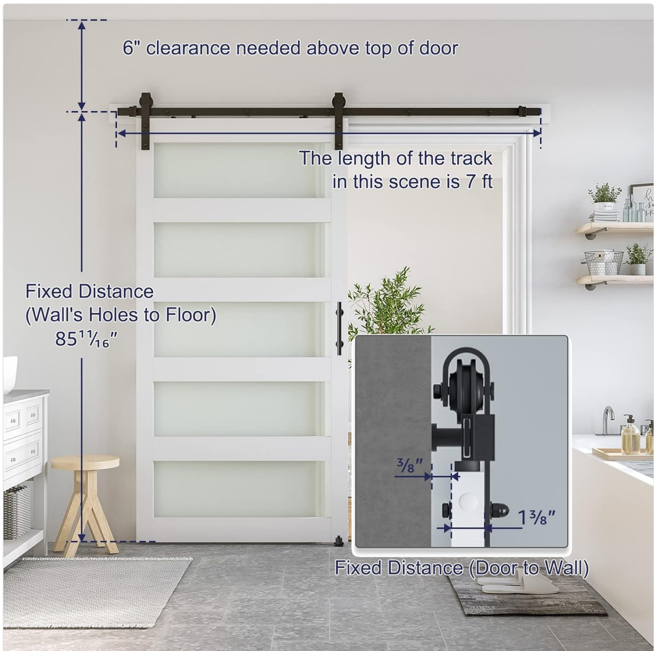
Image: An illustration detailing critical measurements for installation, such as the 6-inch clearance required above the door and the fixed distance from the wall to the door, ensuring proper fit and function.
