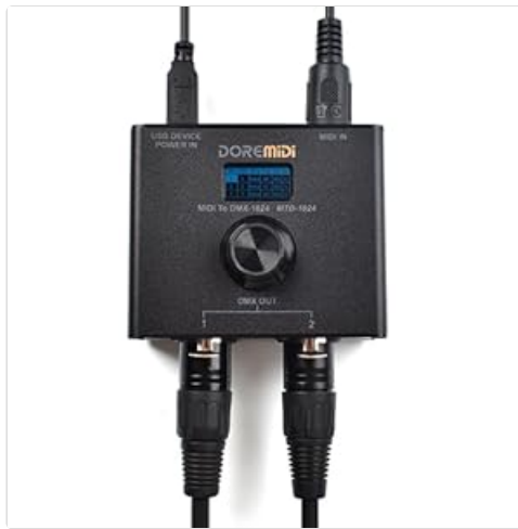
Image: The MTD-1024 controller with both USB and MIDI IN cables connected, ready for operation.
