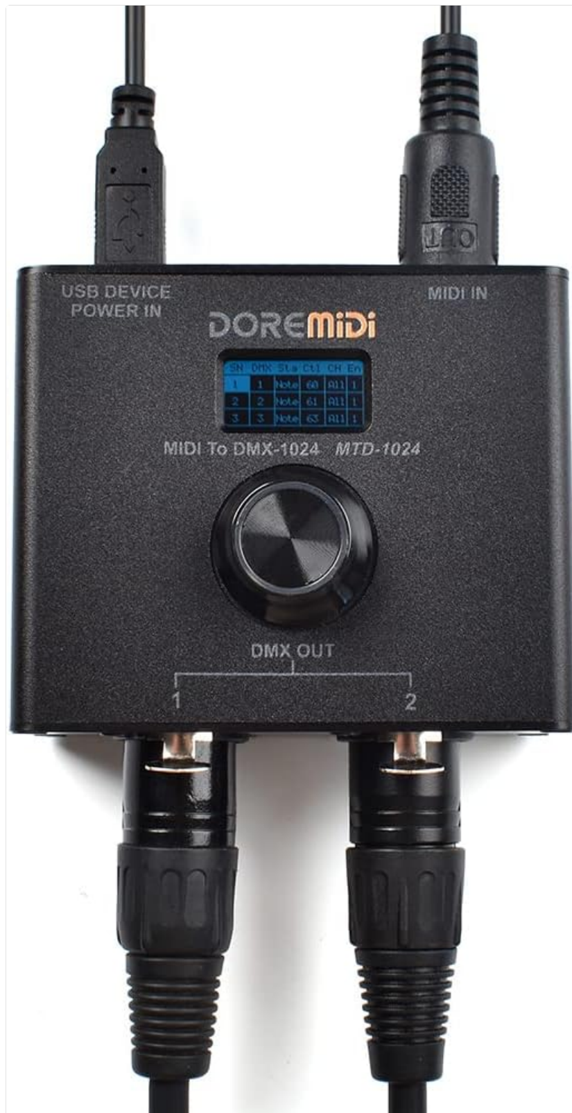
Image: The MTD-1024 controller connected to a computer via a USB MIDI cable, illustrating power and MIDI data transfer.
