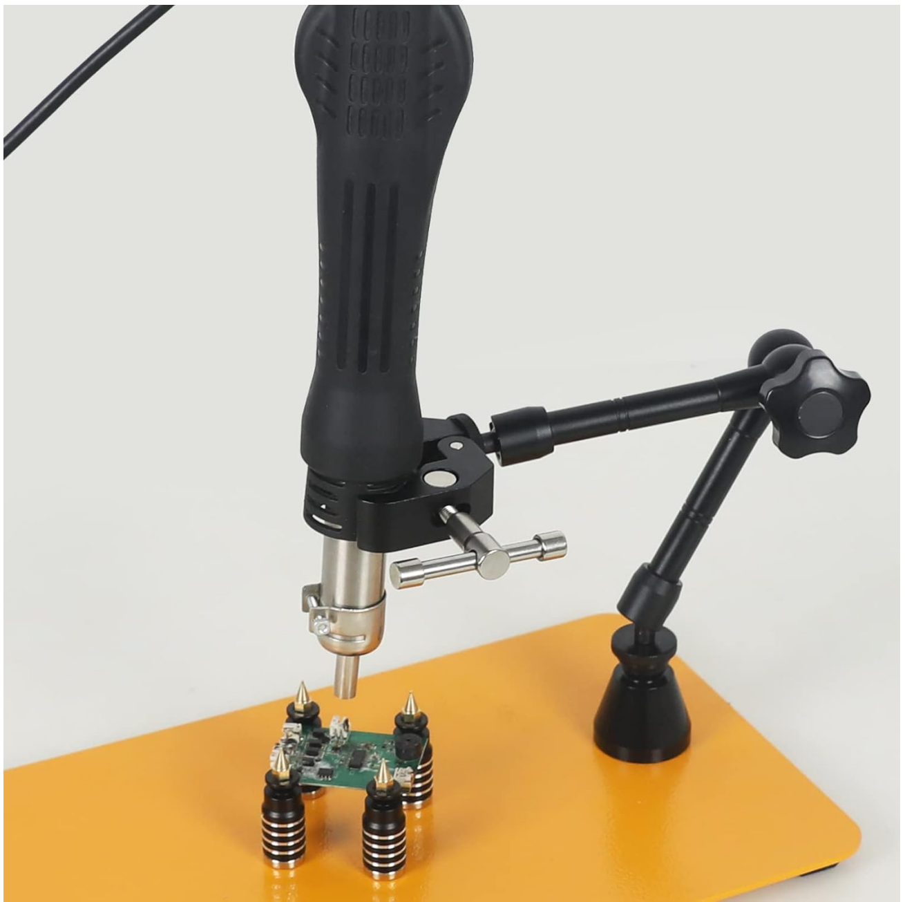
Figure 8: Hot air gun in its holder, demonstrating hands-free operation over a PCB.
