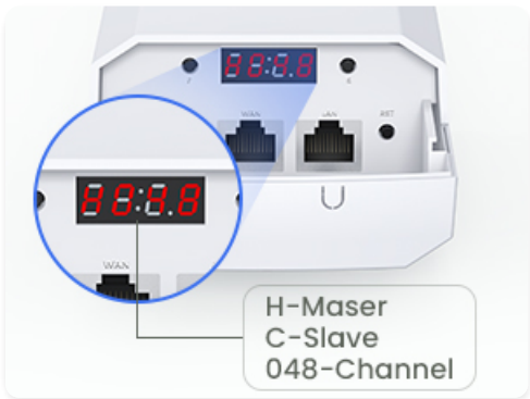
Image: Display showing 'H' for Master, 'C' for Slave, and channel number.
