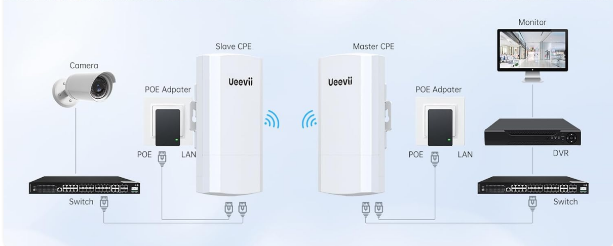
Image: Wireless bridge used for house driveway surveillance.
