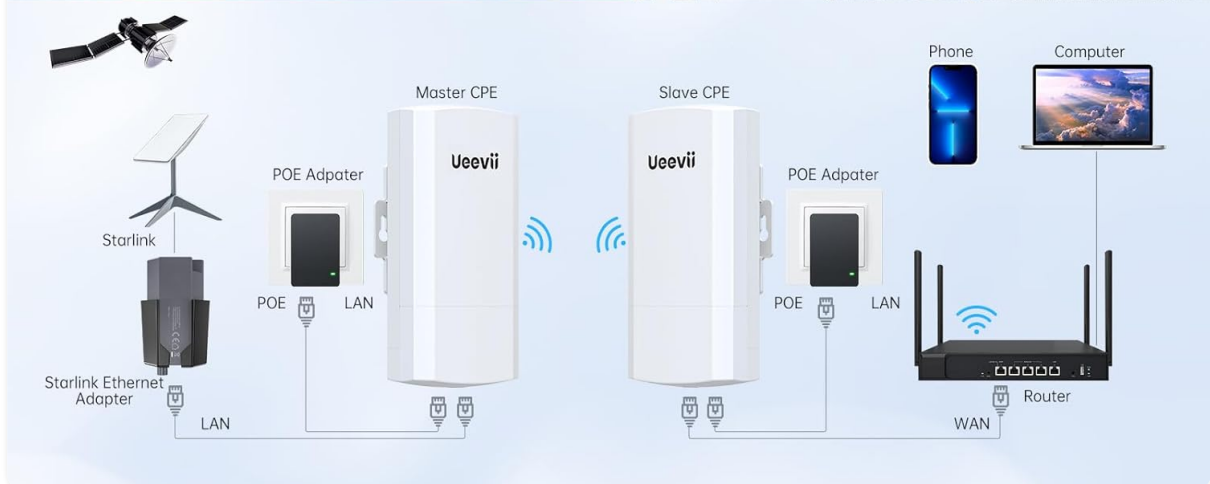
Image: Diagram illustrating how to set up the wireless bridge with Starlink.
