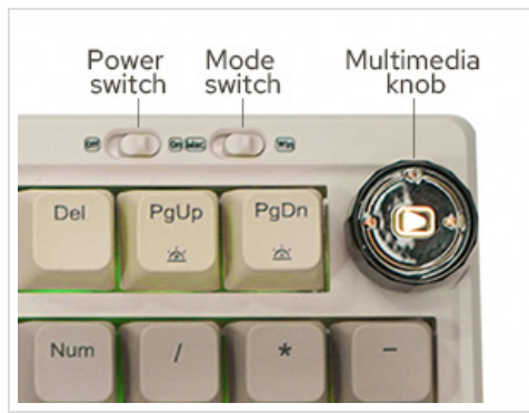
Image: Detail of the power switch, mode switch, and multimedia knob for easy access and control.
