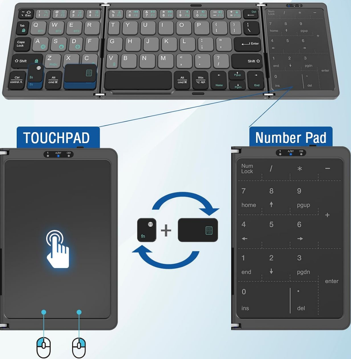
Image: Detailed view of the touchpad and its conversion to a number pad.
