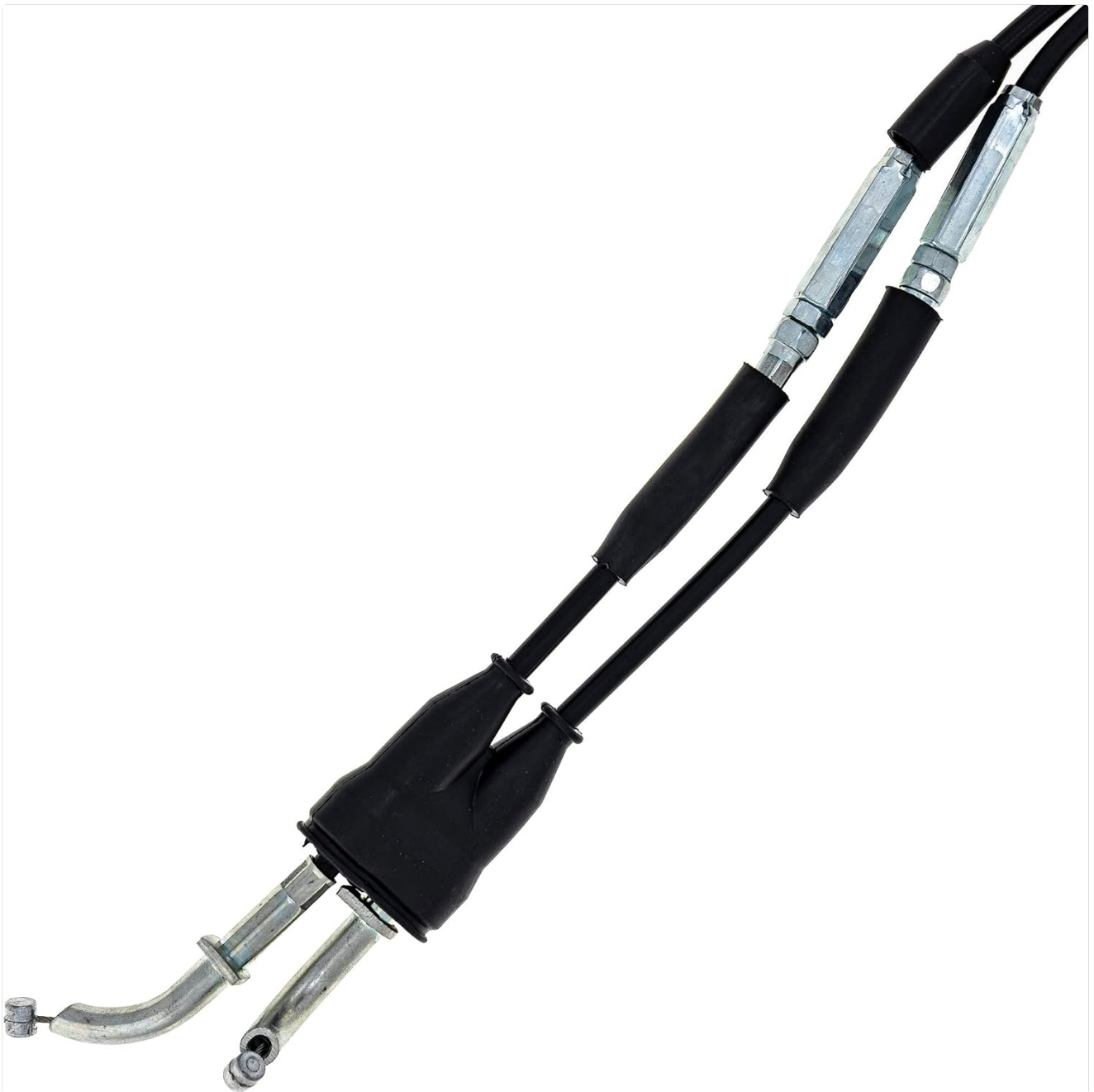
Image: A close-up view of the throttle cable ends, showing the push and pull mechanisms.
