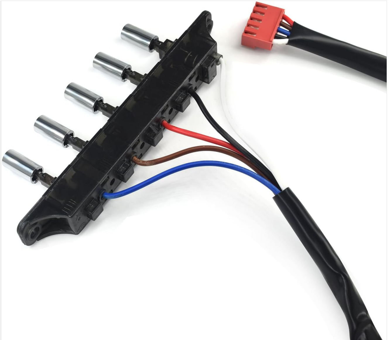
Figure 4: Close-up view of the red connector on the wiring harness, which connects the switch to the range hood's main control system.
