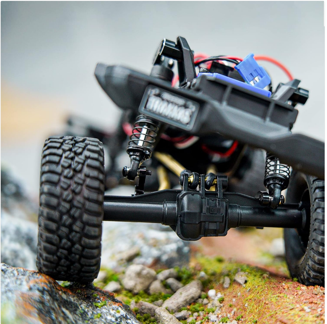
Figure 5.1: RC crawler showcasing enhanced suspension flex with the installed blades.
