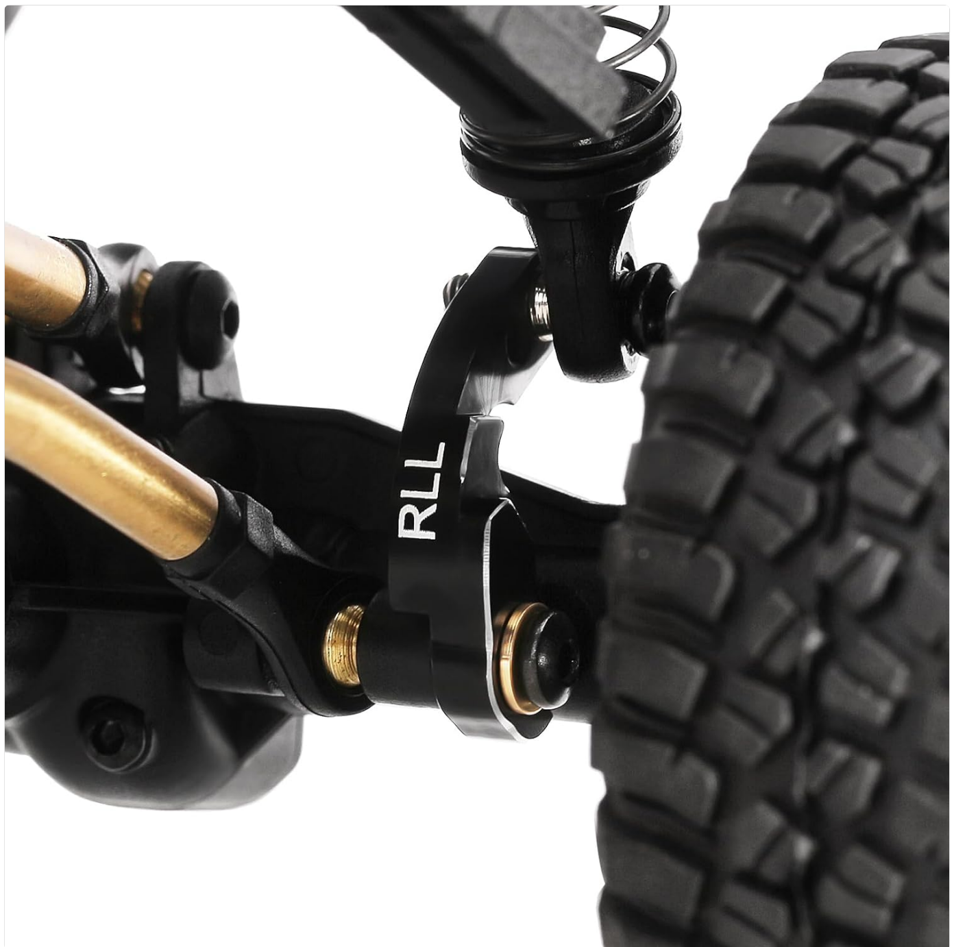
Figure 4.2: Lower flex blade installed on the RC crawler.
