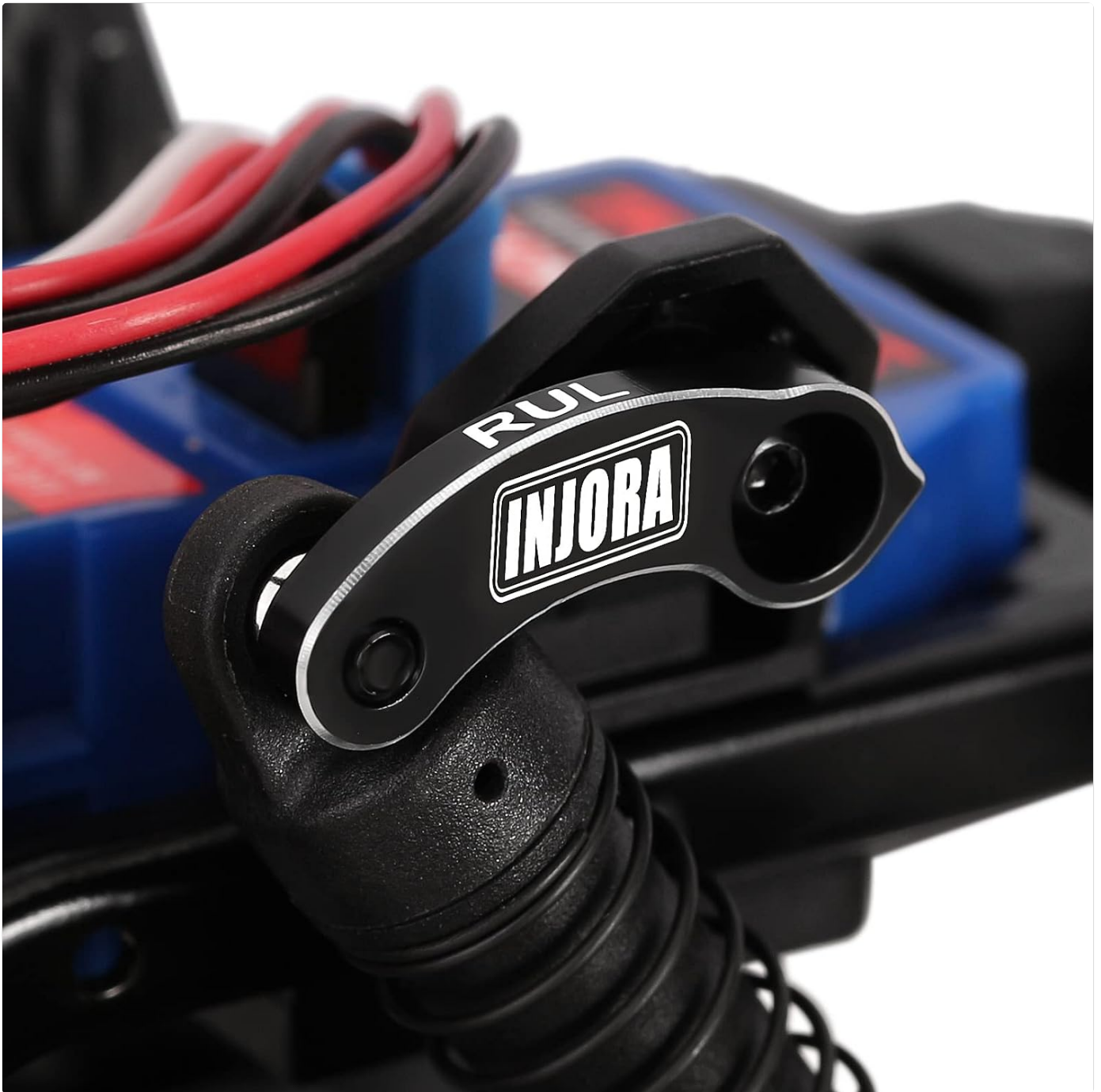
Figure 4.1: Upper flex blade installed on the RC crawler.
