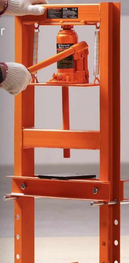
Figure 4.2: The hydraulic jack features a built-in relief valve that automatically releases pressure when exceeding 6 tons, ensuring safe operation and preventing overpressure damage.
