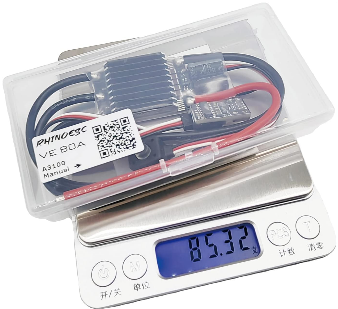
Figure 4: The RHINOESC AM32 Crawler ESC 80A being weighed, indicating its lightweight design.
