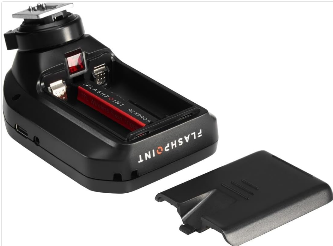
Image 4.1: Battery compartment of the R2 XPro II, ready for AA battery insertion.
