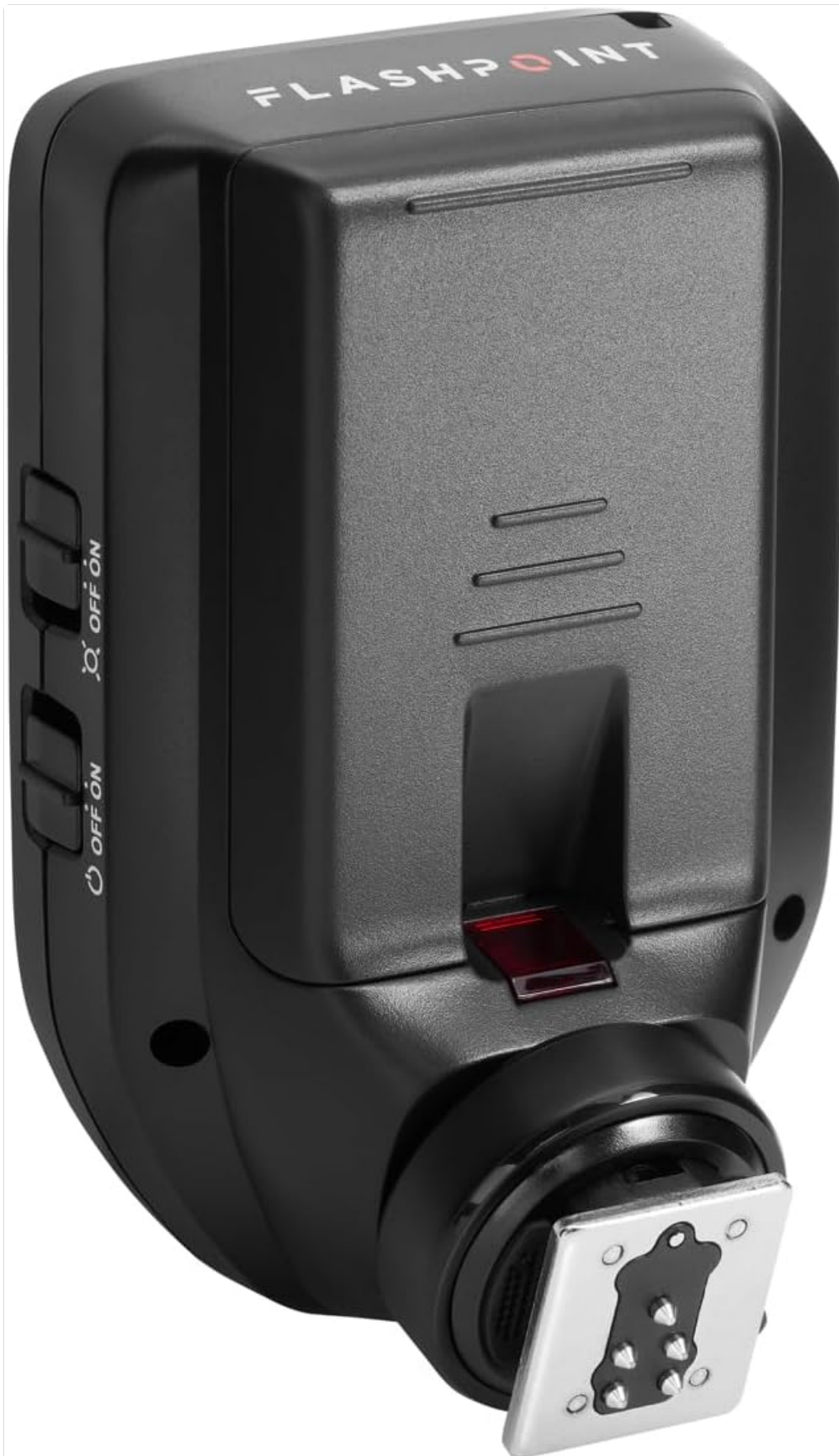
Image 4.3: Side view of the R2 XPro II, indicating the location of the power switch.
